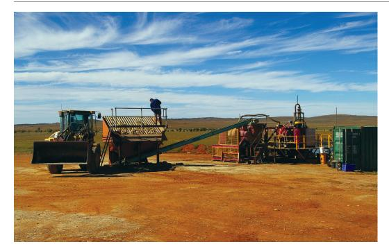
**1-17:** Mineral separation plant used for processing small-scale placer diamond deposits.
