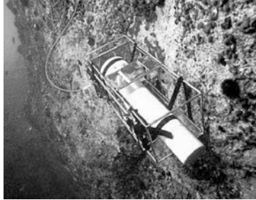
Fig. 2. The gamma-ray spectrometer named KATERINA.
