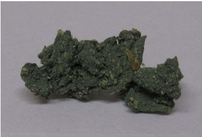
Fig. 4. Odourless and cohesive zeosludge, dried overnight at room temperature.
