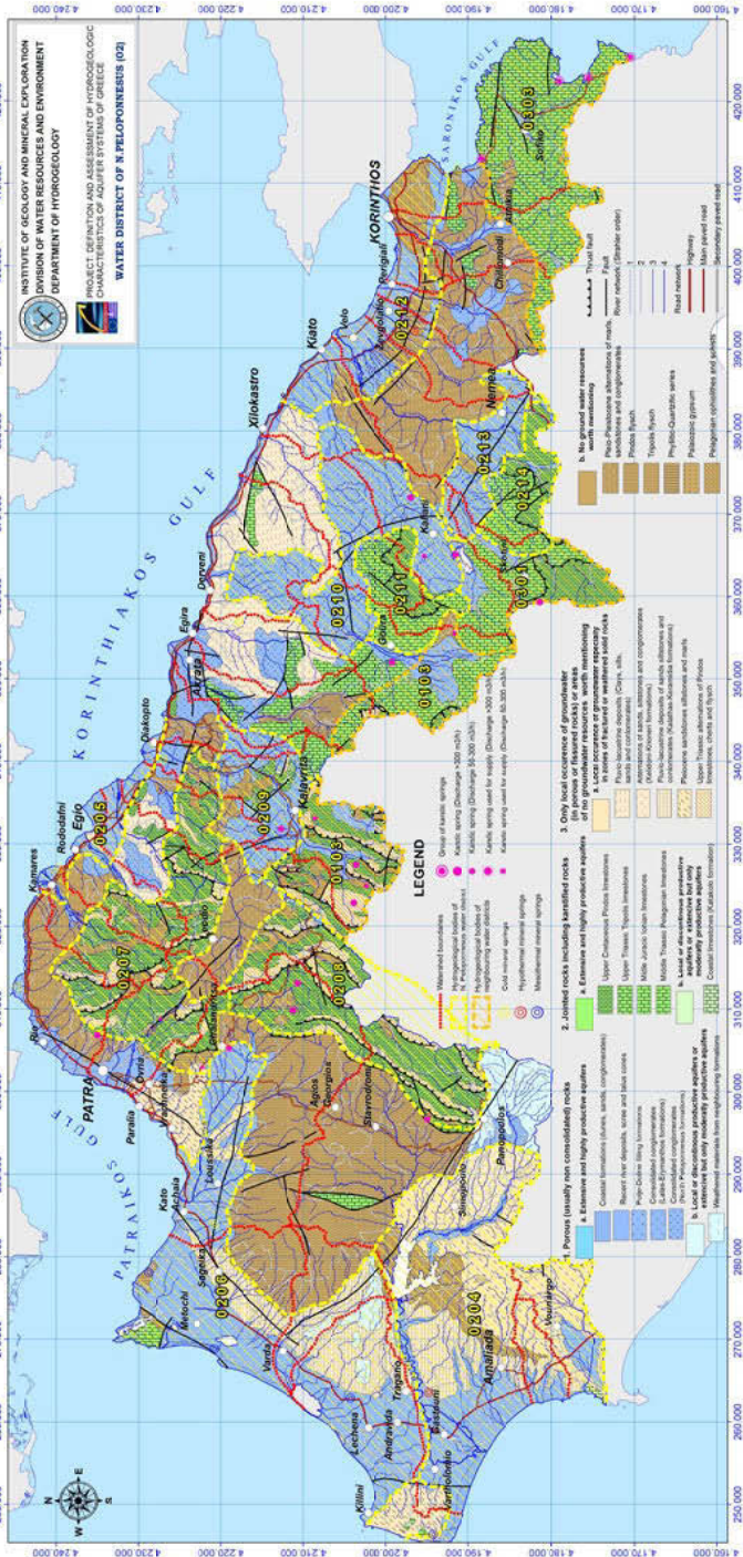
Fig. 1. Hydrogeological map of the study area showing the boundaries of major hydrogeological units as well as the boundaries of the Ground Water Bodies.
