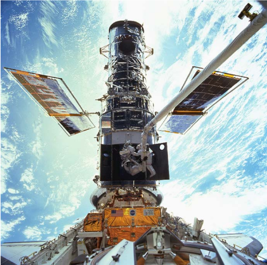
Fig. 48.1 (Color online) Replacement of three Rate Sensor Units during the first EVA of HST SM3A (STS-103) in December 1999
