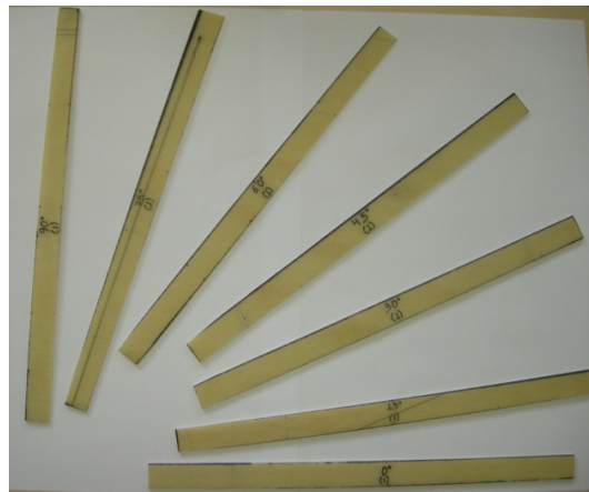
Fig. 5.3 Beam specimens cut from the UD Glass/Epoxy plate at 15^0 increments
