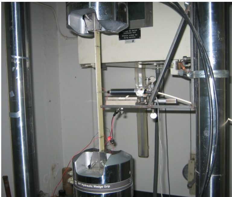
Fig. 5.34 Testing apparatus used in the buckling experiments of Glass/Epoxy beam specimens
