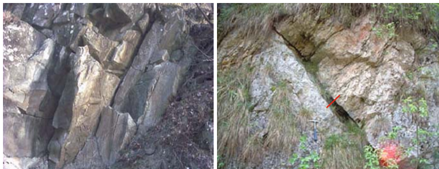
Fig. 1.11 Examples of open discontinuities, with no filling
