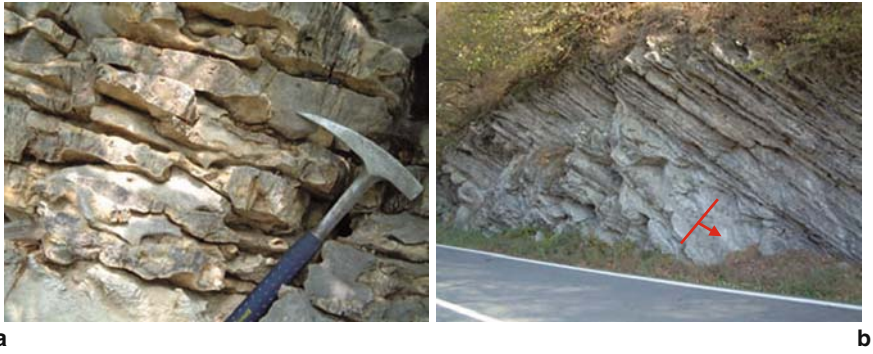
Fig. 1.12 (a) Examples of very undulated joints and (b) example of thickly stratified rock
