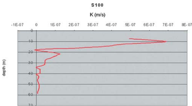
Fig. 6.25 Example of hydraulic conductivity change in depth in a borehole
