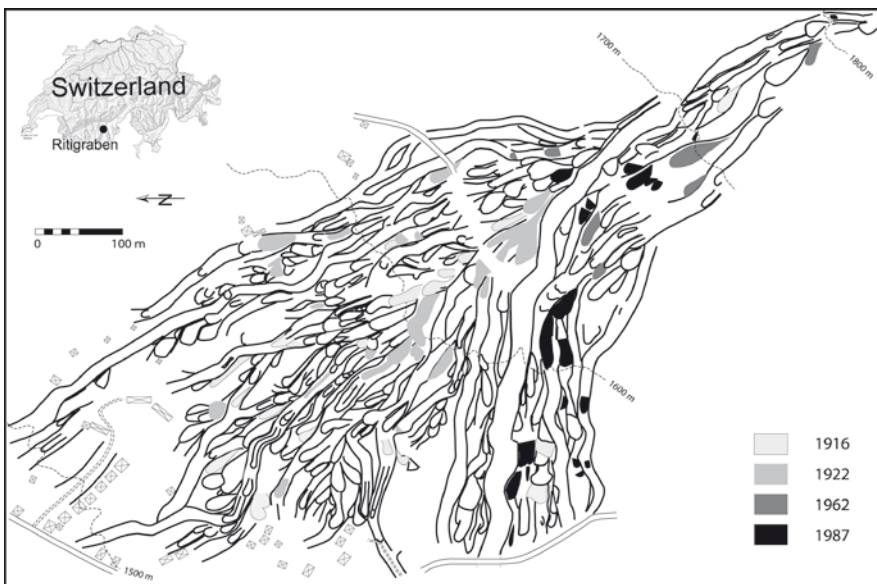
Fig. 8 Deposition of debris-flow material on the intermediate cone during selected events between 1916 and today
