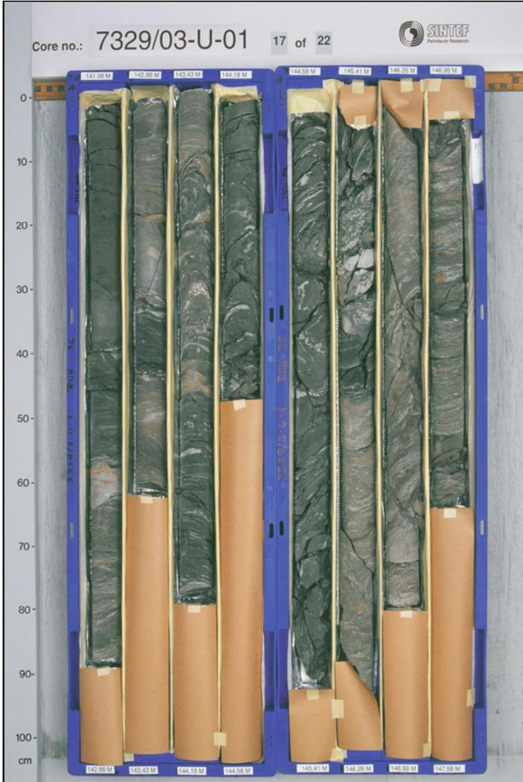
Fig. 8.3 Core photo of core 7329/03-U-01, core depth interval interval 142.86–147.58 m
