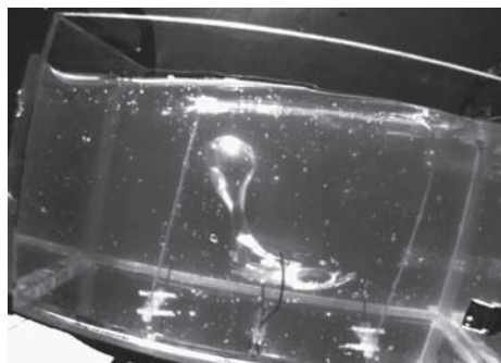
Fig. 6 Gas bubble generated by hydrate dissociation during the pressure release process. The movement of the gas bubble from the dissociated hydrate cavity to the soil surface took approximately 1/15 s (Gidley and Grozic 2008)
