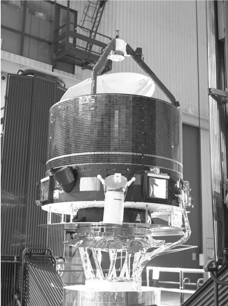
The Giotto spacecraft about to undergo solar thermal tests. The white cylinder in the foreground is the camera baffle, the upward inclined black object at the left is the star mapper. Both would be heavily damaged by dust during the flyby. (ESA)
