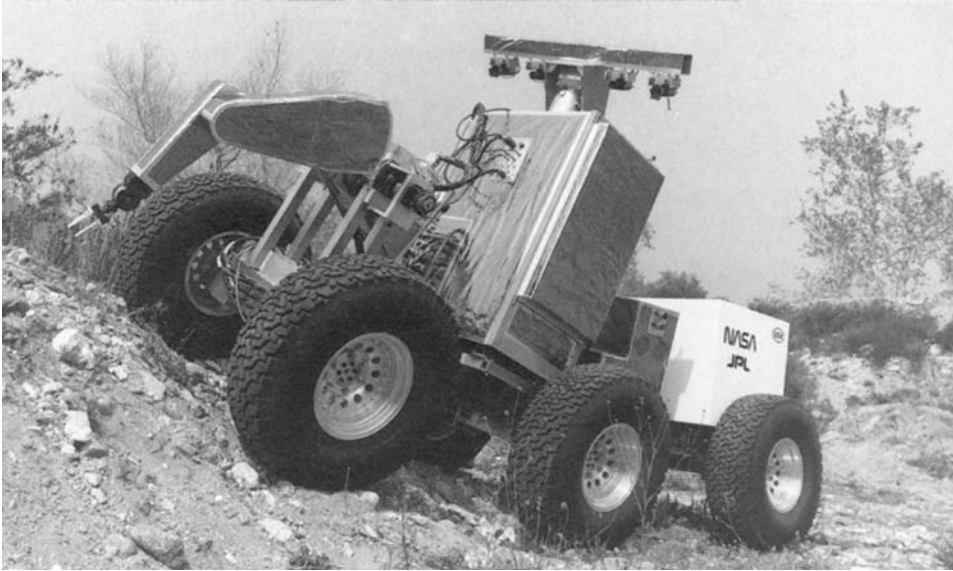
The prototype for the Mars Rover and Sample Return was the huge, three-wheeled rover Robby. (JPL/NASA/Caltech)
