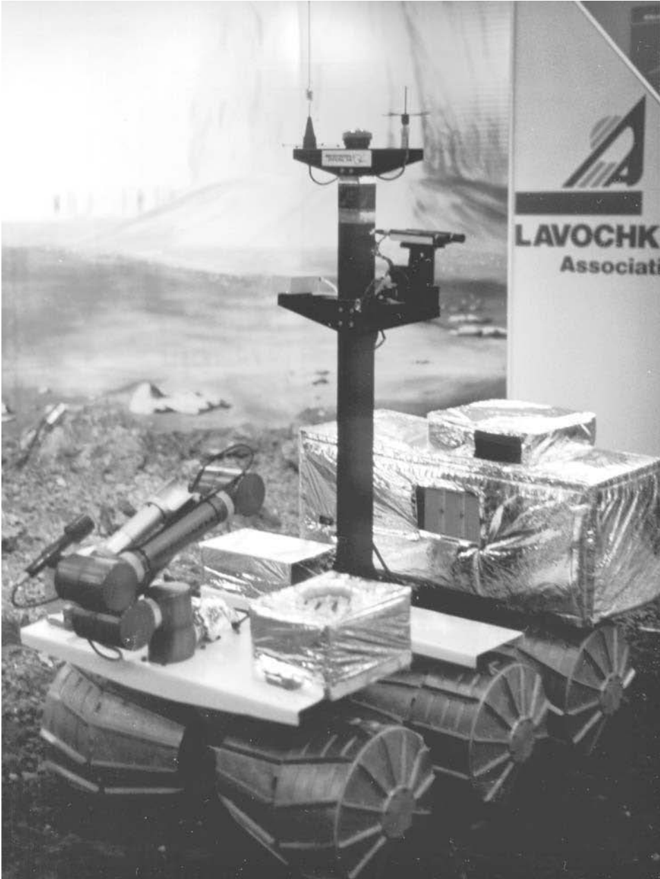
A VNII Transmash prototype Marsokhod with conical-cylindrical wheels which would provide traction in loose soil similar to that of a tracked vehicle.
