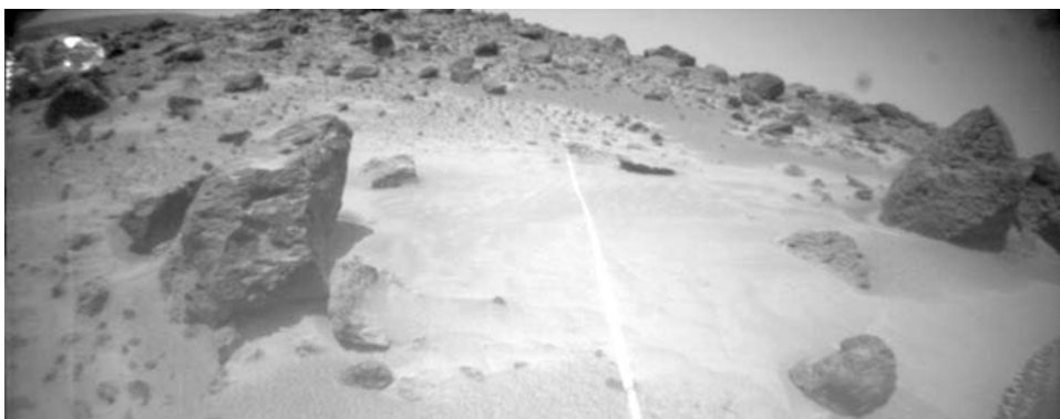
On Sol 8 Sojourner took this picture showing one of its hazard-detection laser stripes. (JPL/NASA/Caltech)
