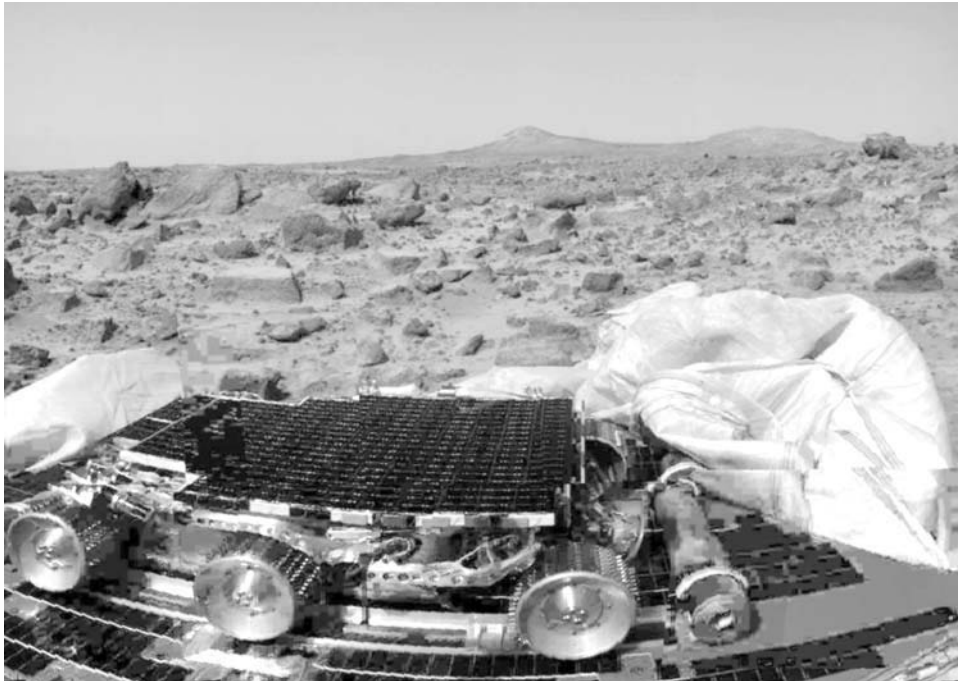
A mosaic taken by Mars Pathfinder shortly after landing. The Twin Peaks are on the horizon, and Sojourner is still in its undeployed configuration on one of the side petals. Note the airbag at right that is obstructing one of the rolled-up exit ramps. (JPL/NASA/Caltech)
