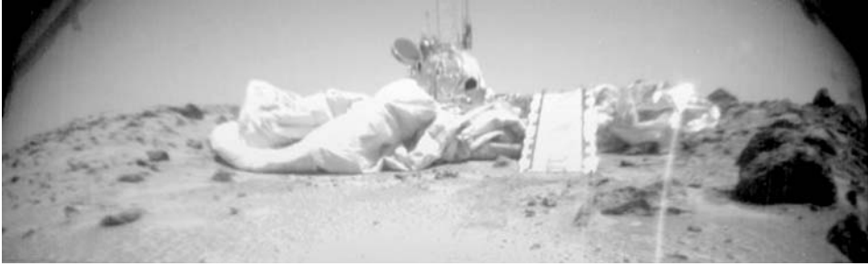
As Sojourner drove away from Mars Pathfinder it provided this view back towards the lander's exit ramp. Most of the lander's structure is obscured by the retracted airbags. (JPL/NASA/Caltech)
