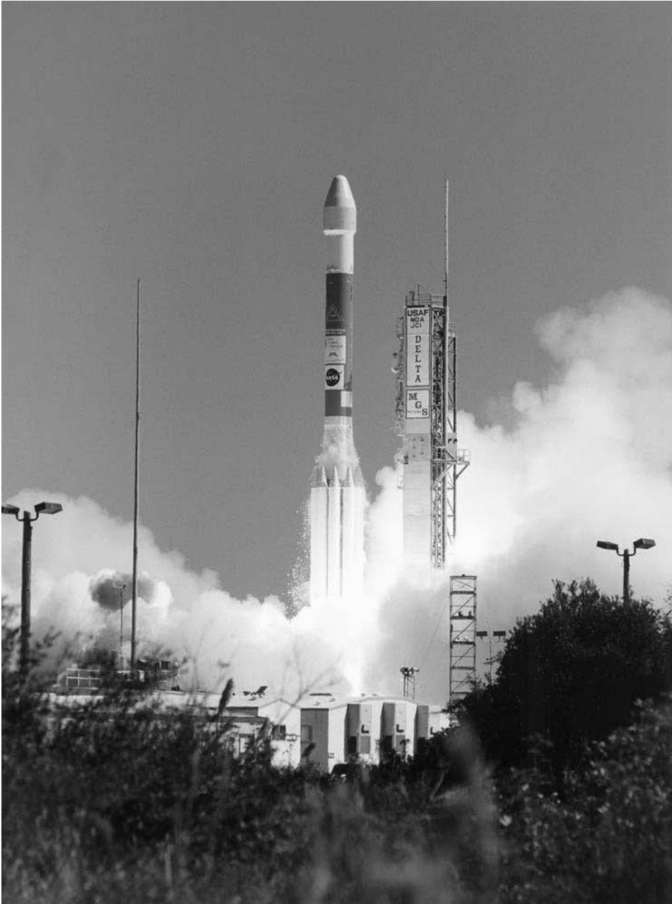
The launch of Mars Global Surveyor on a Delta II rocket. Owing to its relatively low cost, this rocket became the standard launcher for the Discovery and Mars Surveyor missions.
