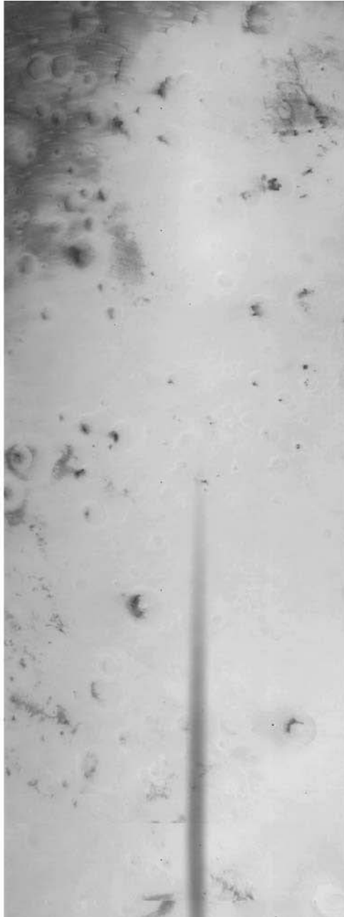
A portion of the final Termoskan swath from Fobos 2. Since Phobos was orbiting Mars at almost the same speed as the spacecraft, the manner in which the image was built up represented the moon's shadow on the surface as a dark cigar-shaped feature.
