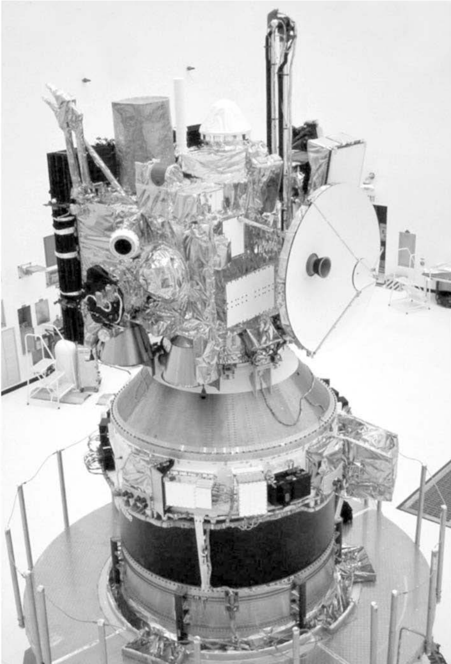
The ill-fated Mars Observer mounted on the TOS stage. The large cylindrical object on the top is the narrow-angle camera.
