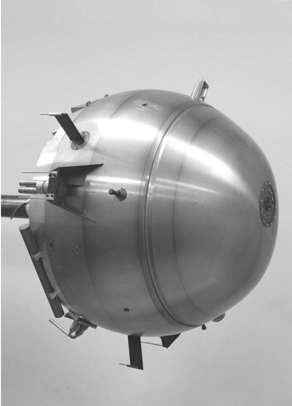
The capsule for the Galileo atmospheric probe being tested in a wind tunnel.
