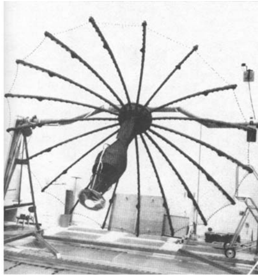
Galileo's high-gain antenna in its deployed configuration during a ground test. The failure of the 'umbrella' to unfurl in flight severely reduced the amount of data that the mission could return.
