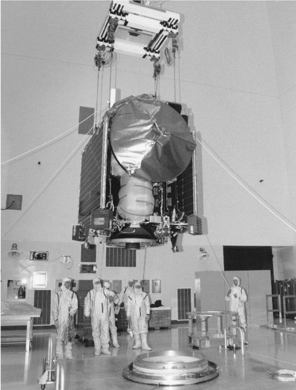
Mars Global Surveyor during ground preparations. This is the high-gain antenna side of the spacecraft. The main engine is visible at the bottom of the 'box'. The only instrument on view is the antenna of the relay experiment which is the white 'rod' at the top.
