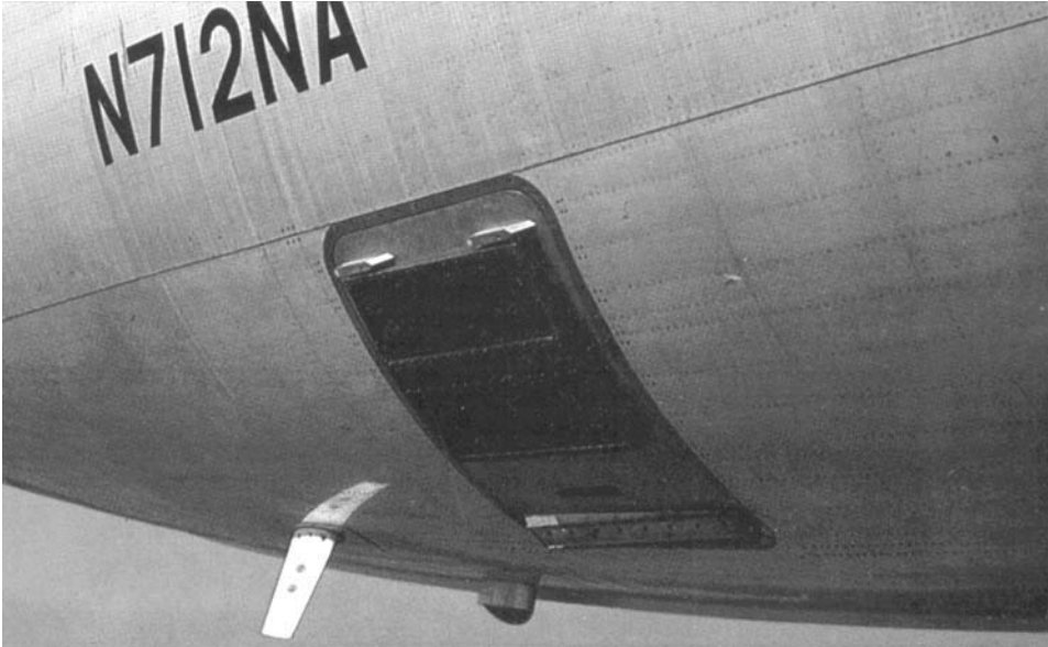
The antenna of JPL's prototype planetary radar protruding from the rear fuselage of the 'Galileo II' airplane prior to a NASA flight over the Guatemalan forest.
