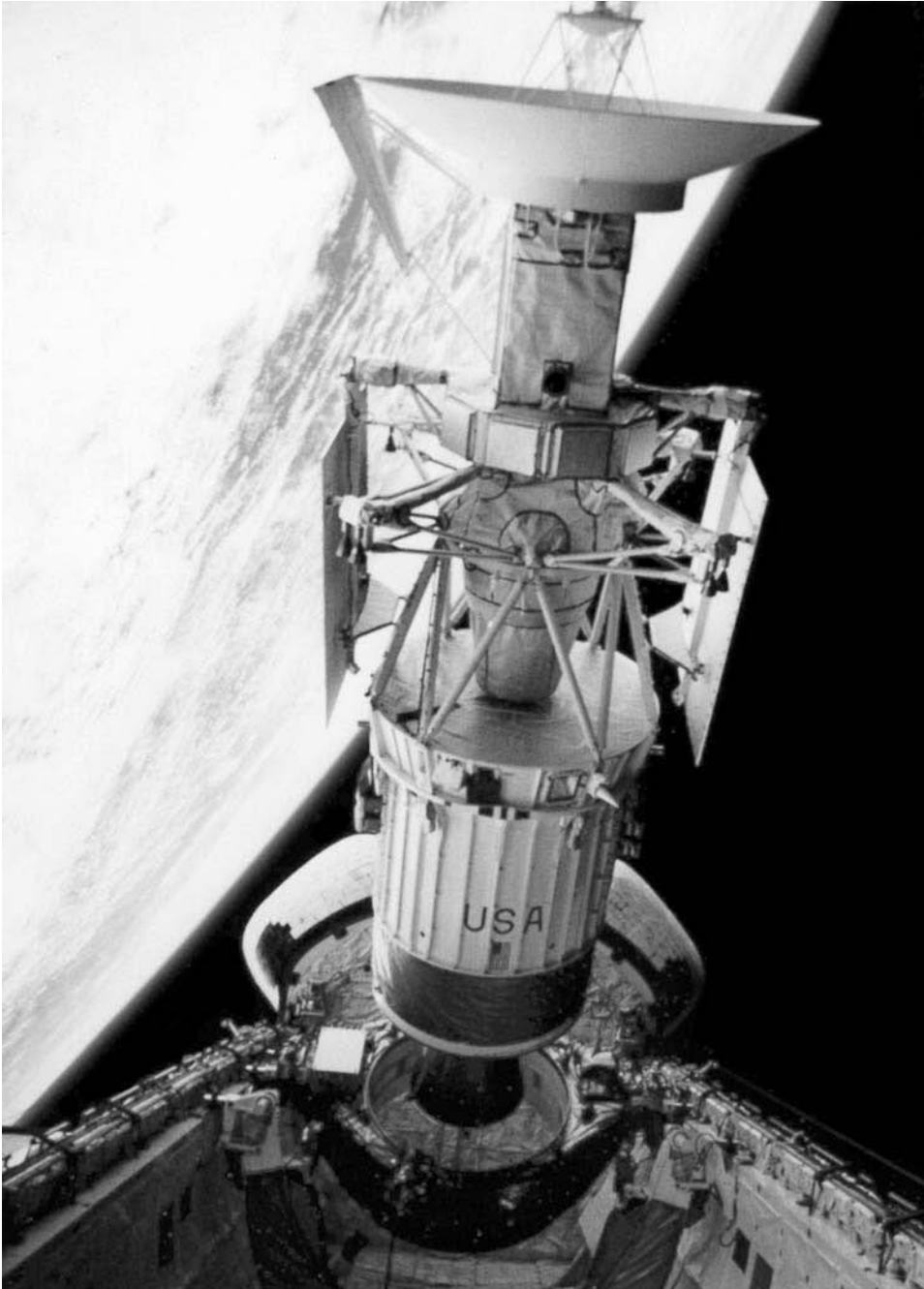
The Magellan/IUS stack leaves its cradle in the cargo bay of Space Shuttle Atlantis.
