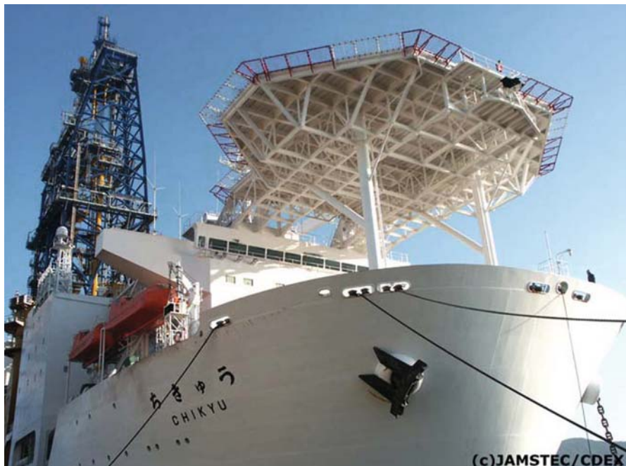
Fig. 1.8 Chikyu, the Japanese deep-sea drilling ship: length 210 m, heights 130 m, gross tonnage 57,087 t, living space for 150 staff and scientists, as well as helicopter deck. Hopefully this vessel will refine our understanding of the state of stress in the oceanic crust
