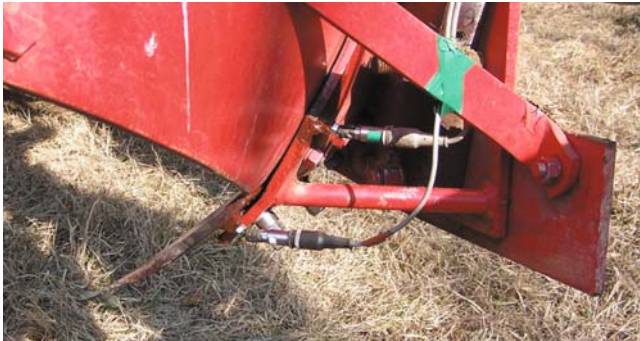
Fig. 3.7 Mouldboard equipped with disc springs
