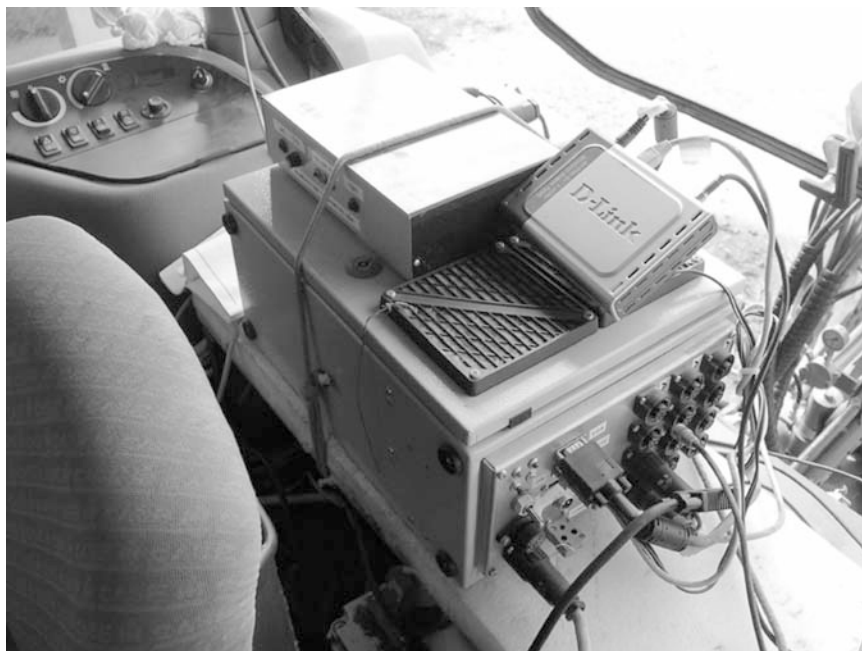
Fig. 10.5 Data acquisition and transmission systems installed on the tractor cab
