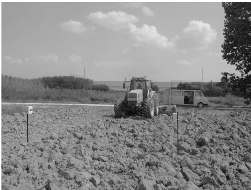
Fig. 10.8 The support unit and a couple of infra-red barriers used to determine the start and the end of the data acquisition
