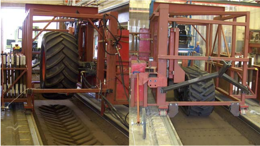
Fig. 6.1 Single wheel/track test apparatus with a tire ( left-hand side ) and a track ( right-hand side )
