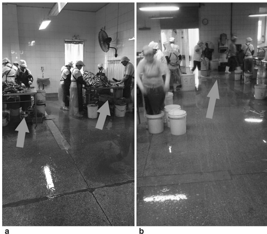
Fig. 10.4 Solid waste drained into wastewater in the preliminary processing step (a) Due to fish that are manually beheaded and gutted, (b) due to parts that are swept into a pipe
