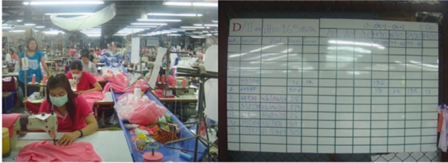
Fig. 9.6 Visual control and dedicated material transport for each worker cell
