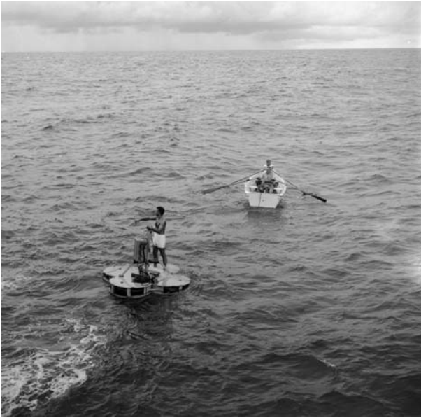
Fig. 3.3 Willard Bascom (above) and Walter observed the hydrogen bomb test, Ivy Mike, at Eniwetok Atoll from a 3 \times 3 foot raft, recording bottom pressure for a possible tsunami. Four truck inner tubes were used for floatation of the plywood raft, which was anchored to the 4500 foot deep seamount by San Diego trolley car wheels. (Willard Bascom on raft , John Isaacs and Monk Hendrix in the rowboat )
