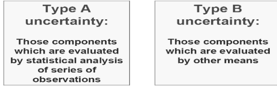
Figure 5. The two methods for the evaluation of uncertainties: Type A and type B uncertainties.
