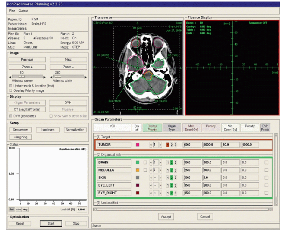
Figure 3. Inverse treatment planning system. In the lower right part of the graphical user interface the dose base constraints can be entered. (Images taken from: Schlegel and Mahr, “3D Conformal Radiation Therapy: multimedia introduction to methods and techniques”, 2nd revised and enhanced edition, Springer Verlag.)
