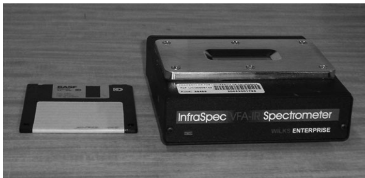
Fig. 12.1 Wilks VFA Spectrometer with ATR crystal, used for collecting mid-IR spectra, compared with a floppy disk
