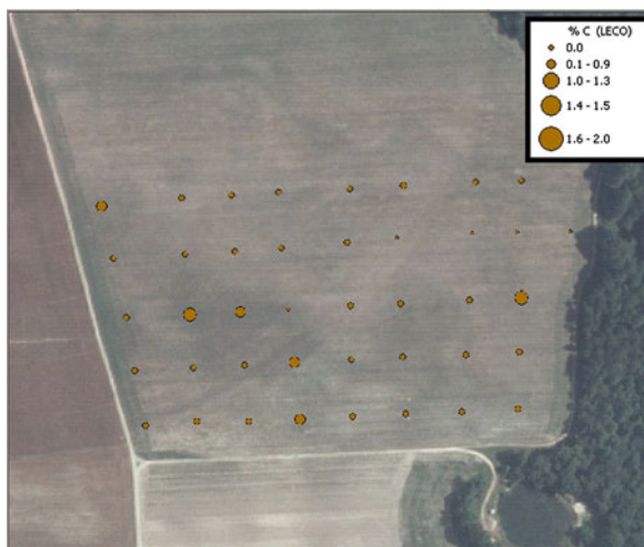
Fig. 14.2 Pattern of soil sampling along transects generated by the tillage-based sensor. The size of the dots indicates relative differences in organic C content
