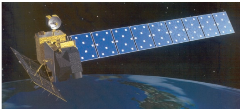
Fig. 3.10 An artist's depiction of the Japanese/JAXA's ALOS Satellite as deployed in space. The three sensors on board are the PALSAR, AVNIR-2 and PRISM (Courtesy of JAXA)
