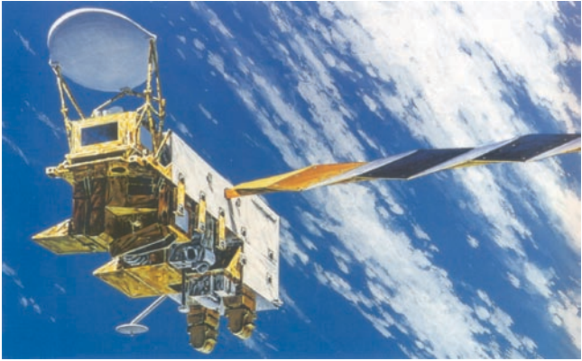
Fig. 3.6 A fully deployed EOS/Aqua satellite with key EOS instruments that include MODIS-A, AMSR-E, and AIRS. Graphic courtesy of NASA
