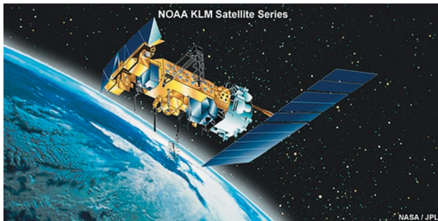
Fig. 3.4 Artist rendition of the NOAA-18 satellite which is a continuation of the KLM series represented by NOAA-15, 16 and 17. The prime sensor is AVHRR-3 which has 6 channels in the visible to thermal infrared regions. The AVHRR series provides continuous global coverage from August 1981 to the present. Graphic courtesy of NASA/JPL and NOAA
