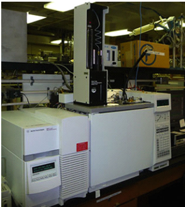
Fig. 5.2 Gas chromatograph/ mass spectrometer in the laboratory of Dr. Stanley Kays. Photograph by Danielle Wedral
