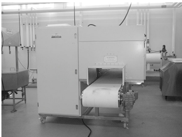
Fig. 17.2 Radiofrequency oven in the University of Georgia pilot plant. Photo by Sara Yang
