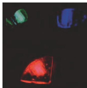
Fig. 9.19 Photograph of the emission states of phosphorescence in glass samples 5 min after the removal of the exciting laser. The \text{Ce}^{3+} -doped calcium aluminosilicate glass sample shows blue light emission. The \text{Tb}^{3+} -doped calcium aluminosilicate glass sample shows green light emission. The \text{Pr}^{3+} -doped calcium aluminosilicate glass sample shows red light emission
