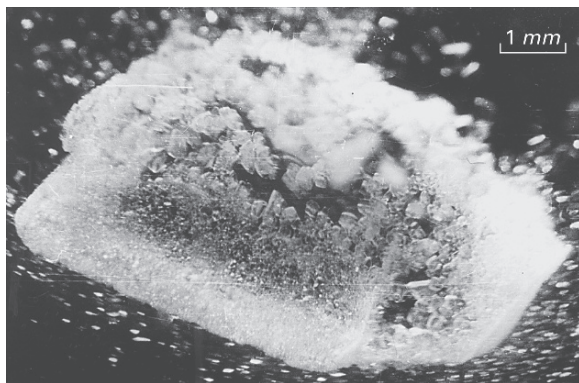
Fig. 1.9 Hollow (box-like, case-like) blurred pseudomorph of K_2Cu(SO_4)_2 \cdot 6H_2O after CuSO_4 \cdot 5H_2O crystals (reaction 1a/22)
