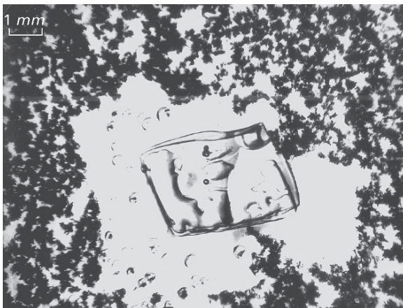
Fig. 1.12 Amorphous (negative) localized automorph after \text{NaNO}_3 formed in a mass of newly produced \text{K}_2\text{Cr}_2\text{O}_7 (reaction II/39 ). Glue film fixes the initial size of protocrystal
