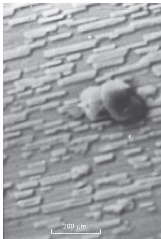
Fig. 3.21 Autoepitaxial excrescences on the growing surface of K_2(\text{Cr,S})O_4 (Photo by I.A. Kasatkin, St. Petersburg University)
