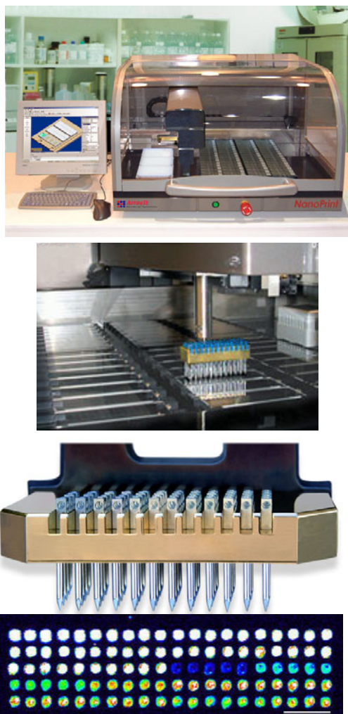
Figure 1. (Top) An example of microarrayer and (middle two panels) its printhead assembled with spotting pins. In the microarray picture, 20 samples were printed in quintuplicate at 200- \mu\text{m} spacing on a glass substrate.(bottom) Samples were mixtures of green- and yellow-dye in arbitrary compositions. Photographs provided with permission from Arrayit Corporation.
