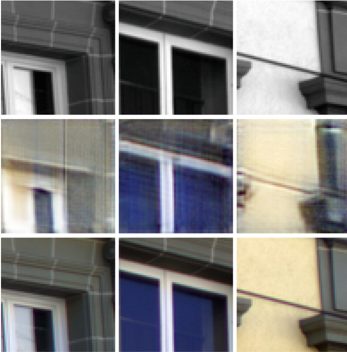
Fig. 3. Set of good results obtained from the proposed approach ( average color angular error: 5.7^\circ ): ( top ) Original NIR patches to be colorized ( 64 \times 64 pixels); ( middle ) Results from the proposed approach; ( bottom ) Ground truth images.
