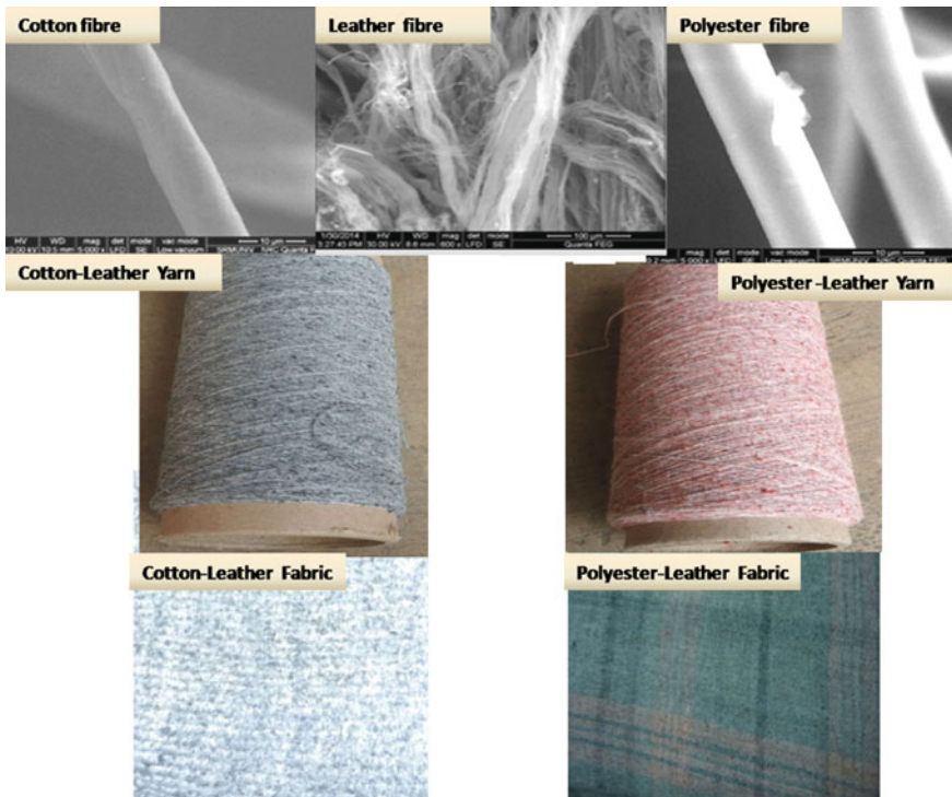
Fig. 1 Leather, cotton, and polyester fibres, yarn, and fabric from blended fibres (Senthil et al. 2014)
