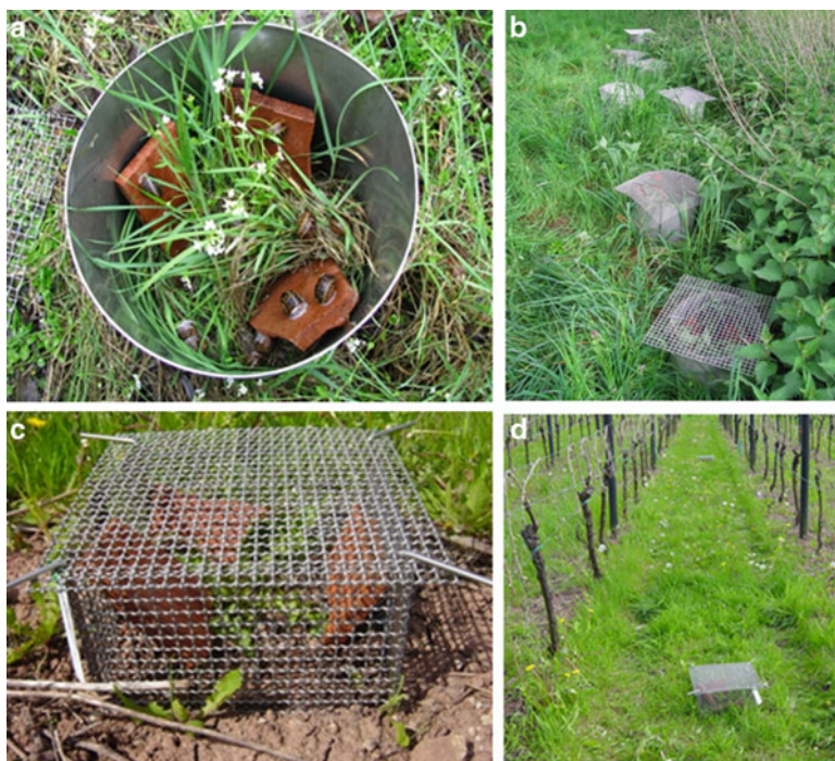
Fig. 23.3 (a, b) Microcosms used to assess bioavailability of MTE on field sites (Scheifler et al. 2003a; Gimbert et al. 2008b; Fritsch et al. 2011; Pauget et al. 2013a, b). (c, d) Wired microcosms (25 × 25 × 15 cm, mesh size of grid: 1 cm) closed by a stainless steel grid of 30 × 30 cm adapted to study the fate and effects of pesticides sprayed in a vineyard (Druart et al. 2011b)
