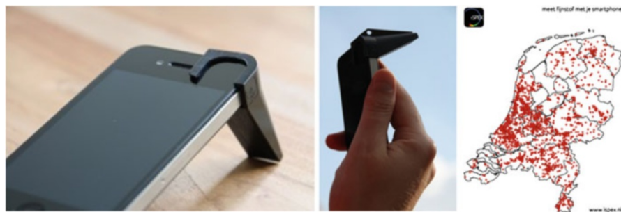
Fig. 50.9 Example of using crowd sourcing to collect data on atmospheric particle concentrations. The technology was developed as the Spectropolarimeter for Planetary EXploration (SPEX) and designed to measure aerosol and cloud particles in the atmospheres of planets within the solar system. This technology was simplified and miniaturized to a setup-module for a smartphone supported by an app ( www.ispex.nl ). The goal is to involve 10,000 users in this citizens' science network in The Netherlands
