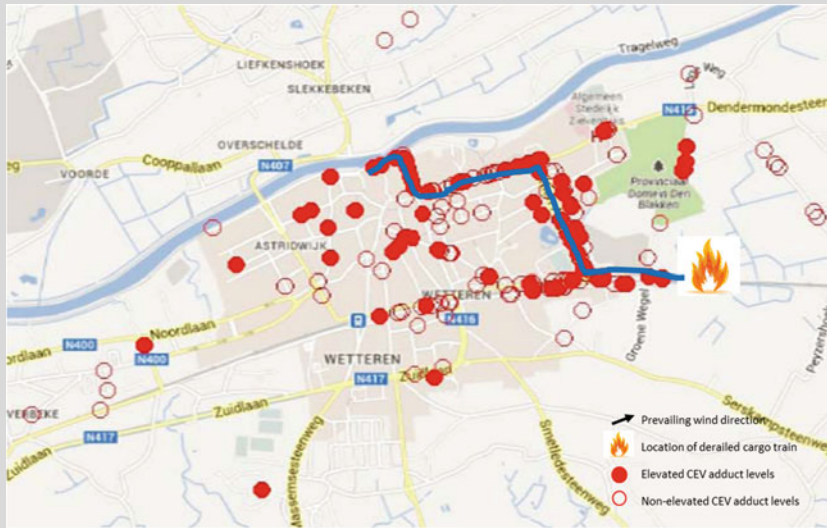
Fig. 54.2 Pattern of elevated CEV-Hb adducts levels measured in blood of inhabitants of Wetteren. The blue line indicates the main sewer system between the incident location and the river Schelde. Used cut-off values of 200 /g (smokers) and 10 pmol/g (non-smokers) (Source: WIV-ISP, Brussels)
