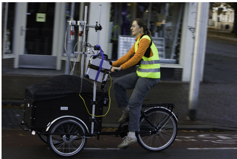
Fig. 50.8 Equipment for measurement of ambient particulate matter for estimation of the exposure of commuters to traffic fumes in The Netherlands (Photo: Bas de Meijer)
