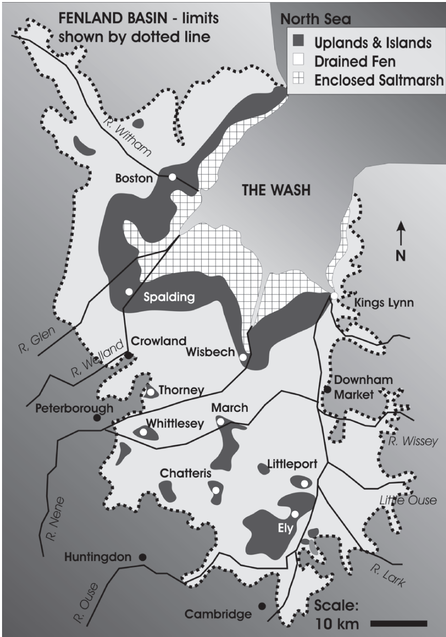
Figure 15 Progressive and cumulative embankment and drainage in the Fenland Basin, in relation to the saltmarshes of the Wash, eastern England. Redrawn from interpretative material at the Flag Fen Bronze Age Centre, Peterborough, UK http://www.flagfen.com/ . See also Brew & Williams (2002) for details of the changes in the extent of the shoreline before embankment. Note Joan Blaeu’s map of 1643 also shows the extent of the fens in relation to the ‘uplands’ particularly well
