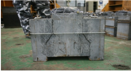
Fig. 8. Failure of UHPFRC precast joint (Cast-in-place joint)
