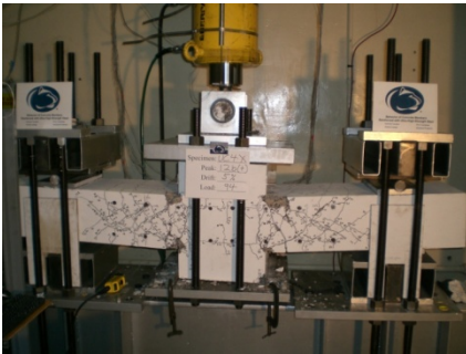
Fig. 5. Specimen #2 at 5% drift
