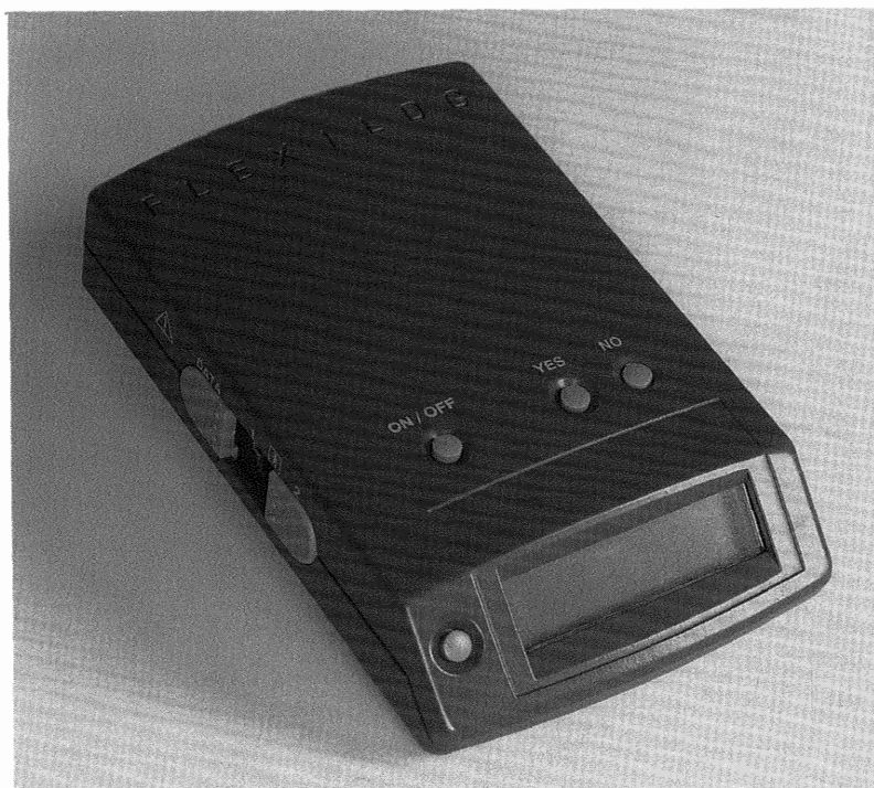
Fig. 4.2 Flexilog 2000 pH recorder (Oakfield Instruments).
