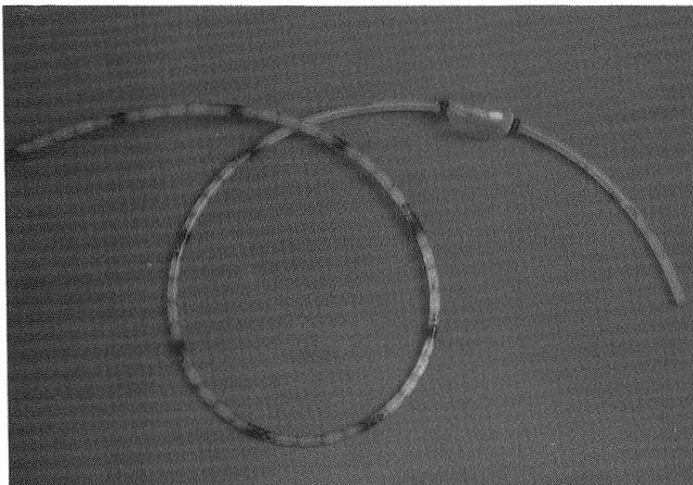
Fig. 10.5 An inflated 3 cm long latex balloon attached over one of the recording channels of a standard Arndorfer multilumen oesophageal manometry catheter.
