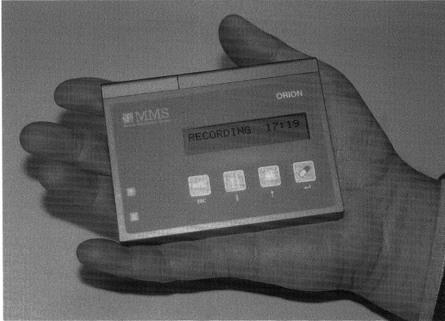
Fig. 4.3 Orion pH recorder (Medical Measurement Systems).
