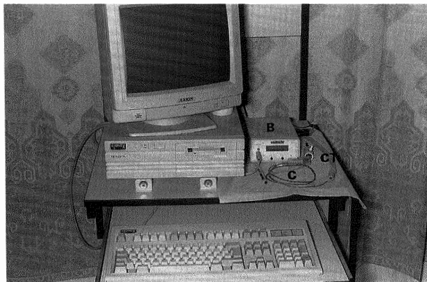
Fig. 3.10 The system for oesophageal manometry using solid state catheter (C) and a personal computer (PC). The calibration tube is shown (CT). The interface box (B) links the catheter to the PC for data acquisition. The PC enables data display, analysis and hard copy printout.
