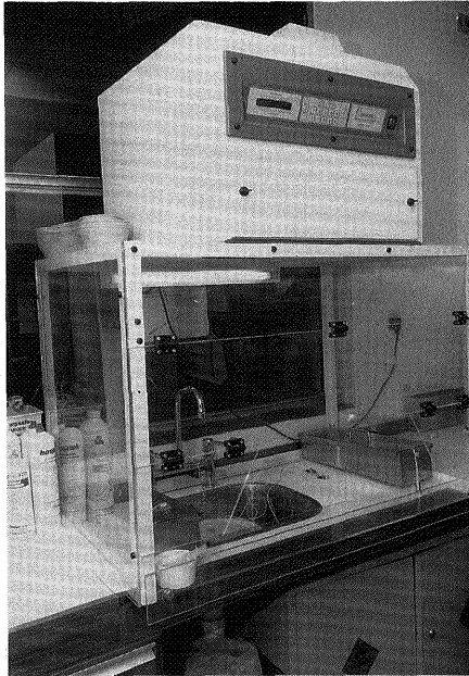
Fig. 3.12 The fume cabinet is used for disinfection of the catheters and to house the glutaraldehyde containers. The filter is contained on top of the cabinet which both filters and recirculates the air.
