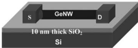
Fig. 5.6. A back-gate nanowire transition using Ge nanowire as channel
