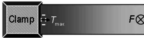
Fig. 8.15. Top view of clamped-free cantilever with two longitudinal and two transverse piezoresistors located in the stress concentration region
