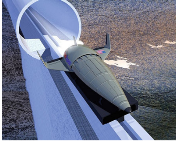
Fig. 7.25 A prior concept for a horizontal launch assist system based on superconducting maglev tech, but at far lesser velocity: MagLifter [19]
