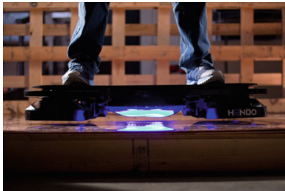
Fig. 7.16 General view of an active type magnetic hover board having 2 magnetic wheels [13]
