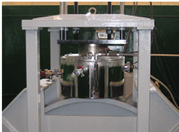
Fig. 4.10 Roller rig for experimentation of levitation and drag forces
