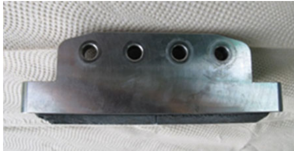
Fig. 6.44 Landing skid made of sintered alloy
