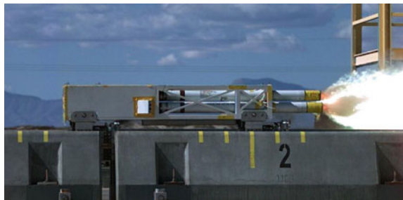
Fig. 7.27 Superconducting maglev track for flight tests [21]
