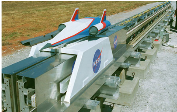
Fig. 7.24 A track on test model scale for lower velocity magnetic launch assist [18]
