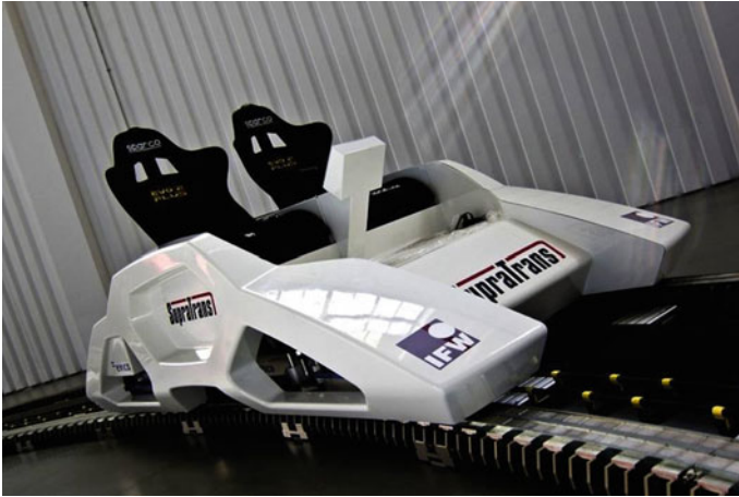
Fig. 4.5 The maglev vehicle, named SupraTrans, using the flux pinning effect [2]
