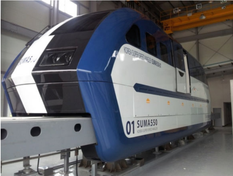
Fig. 5.10 General view of an experimental maglev vehicle with the electromagnets for suspension and guidance [2]
