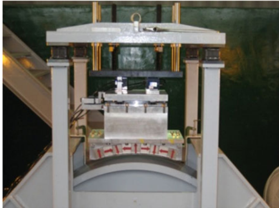
Fig. 3.10 Electrodynamic levitation with a moving Halbach array magnet [3]
