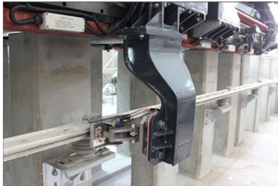
Fig. 6.45 Configuration and location of power rails
