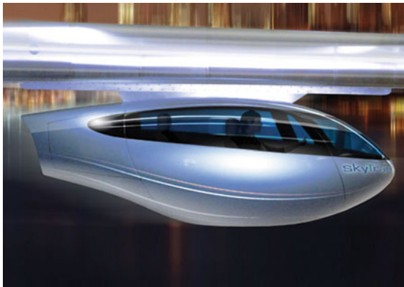
Fig. 1.9 PRT (Personal Rapid Transit) using electromagnets and LIMs [5]
