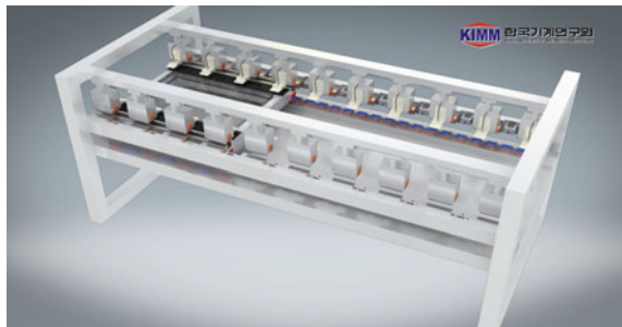
Fig. 7.9 General view of the passive tray conveyor system
