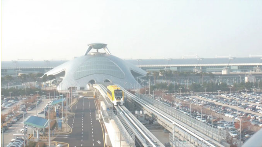
Fig. 6.22 ECOBEE on the 6.1 km long Incheon International Airport Urban Maglev Demonstration Line
