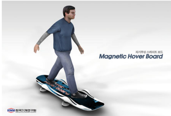
Fig. 7.15 Conceptual illustration of an active type magnetic hover board having 4 magnetic wheels
