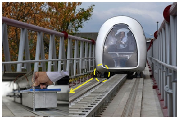
Fig. 4.7 Maglev-Cobra using flux pinning effect [5]
