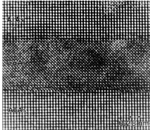
Fig. 3.32 High-resolution TEM of an AlAs/GaAs double heterostructure. The dark and bright points are correlated with single rows of atoms [3.28]
