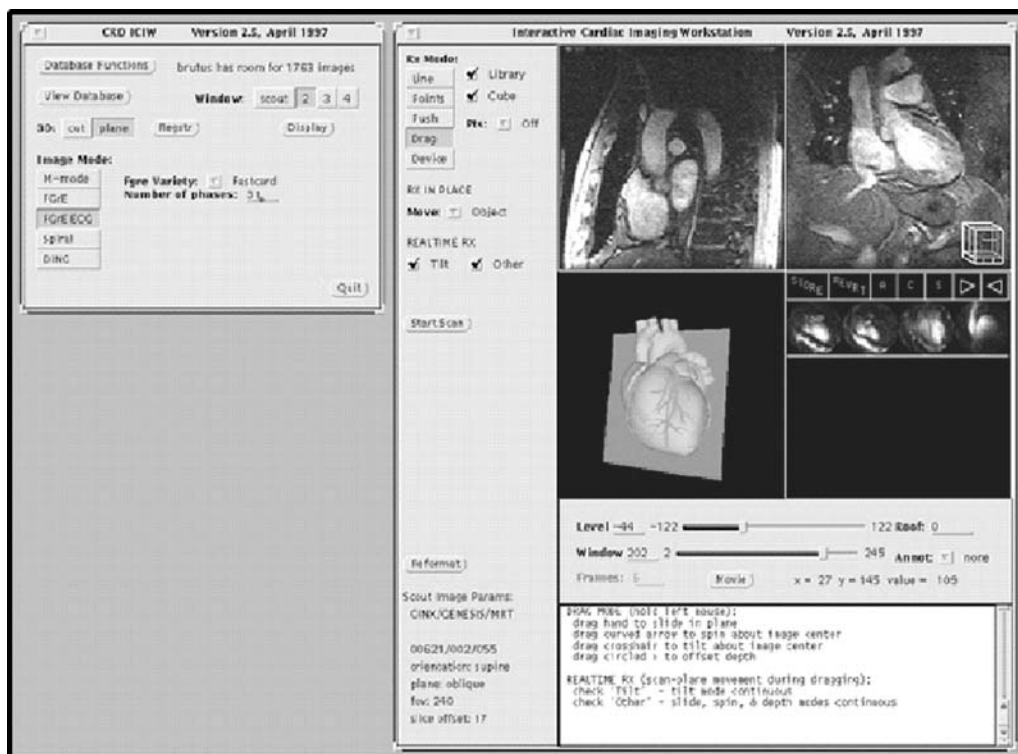
Fig. 1. Real-time interactive software interface. The two cardiac MR images on the upper right of the panel represent two orthogonal slice prescriptions that serve as scout images for later prescriptions. The drawing of the heart shown in the lower left panel serves as an anatomic landmark that shows the position and orientation of the slice. Using mouse or trackball control, the slice can be altered in real time and imaging parameters such as slice thickness and field-of-view can be defined.
