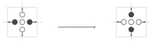
Fig. 13.2 Example of a possible interaction of particles at a node \mathbf{r} ; filled dots denote the presence of a particle in the respective channel. Arrows indicate channel directions
