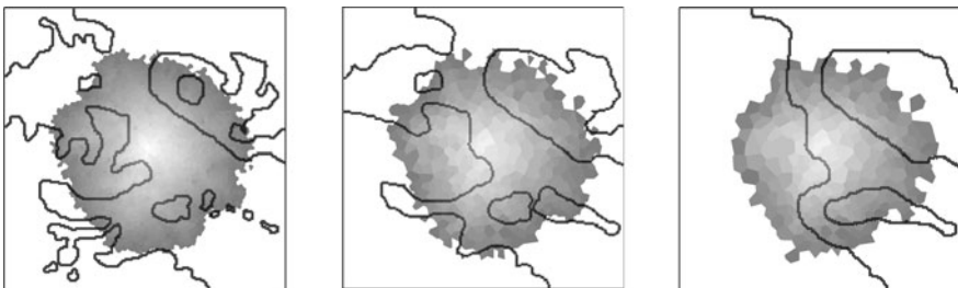
Fig. 4.10 Activation times for a single simulation of a homogeneous propagation rule over three levels of a heterogeneous cellular structure. The time to activation is represented by the difference in shading (from light to dark). The cellular structure is as given in Fig. 4.7. Isotropic propagation is expected
