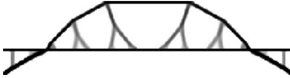
Fig. 14.7 Optimal 2-D topology of compression bridge
