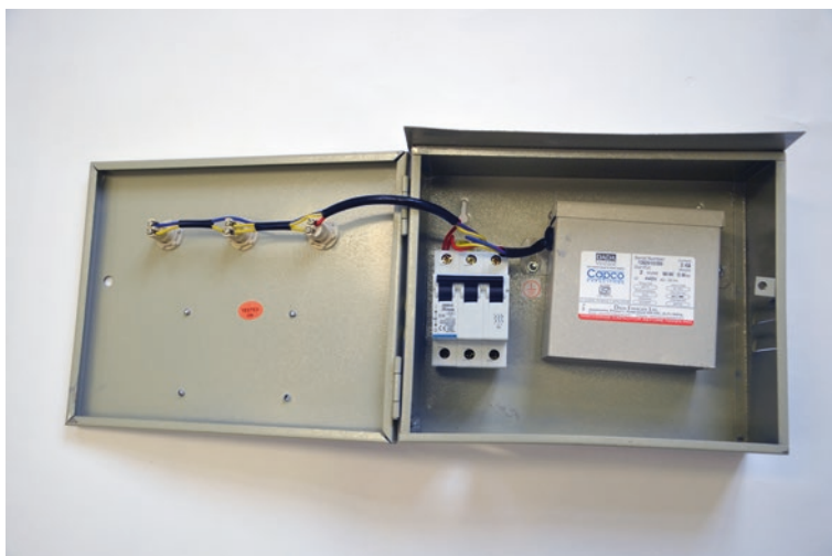
Fig. 7.11 Redesigned capacitor box with miniature circuit breaker, used in phase II. Source Malte Müller
