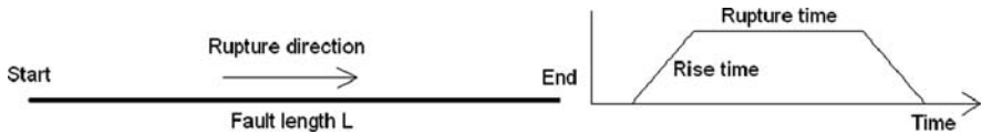
Fig. 7.41 Schematics of a rupturing fault with length L ( left ) and the resulting time pulse also taking rise time into consideration ( right ), see text
