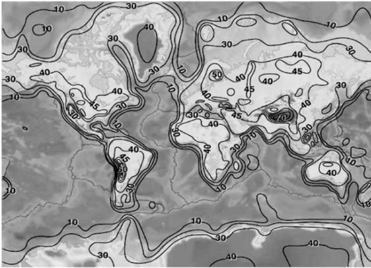
Fig. 2.2 Contour map of thickness of the Earth's crust. The contour interval is 10 km except for the continents where contour 45 km also is included. Figure from http://earthquake.usgs.gov/research/structure/crust/index.php
