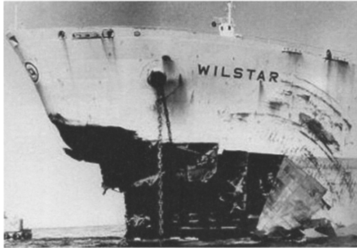
Figure 2.19. Impact of a freak wave on the Norwegian freighter Wilstar in 1974. Credits: ESA/DLR.
