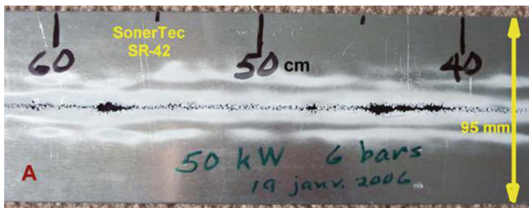
Fig. 7.11 Erosion of a 1.5 mm aluminum alloy plate during a 5-min exposure in model SR-42 (50 kW)
