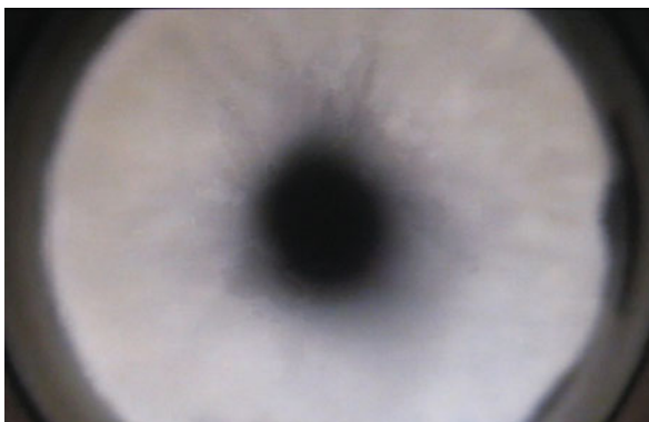
Fig. 7.5 Cavitation zone in the low-power SR-31 sonoreactor. Tube diameter: 75 mm
