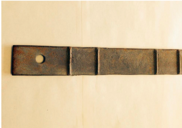
Figure 14.1 Representation of steel strip reinforced wall and detail of ribbed galvanized strip.
