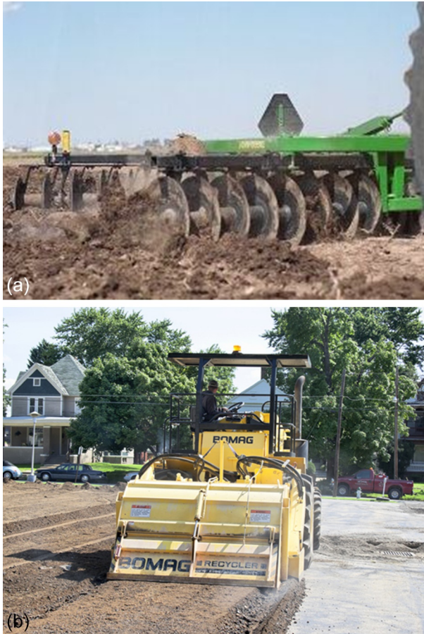
Figure 11.8 Typical surface mixing equipment. (a) Disk harrow (Courtesy of EPA). (b) Recycler/traveling mixer (Courtesy of Bomag).
