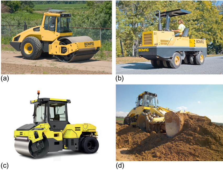
Figure 5.7 Photographs of typical shallow compaction rollers. (a) Smooth drum roller (Courtesy of Bomag). (b) Pneumatic tire roller (Courtesy of Bomag). (c) Combination roller photo (Courtesy of Dynapac). (d) Sheepsfoot/padfoot roller (Courtesy of Bomag).
