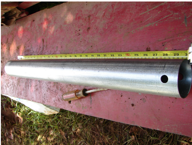
Figure 3.21 Thin-walled Shelby tube sampler.
