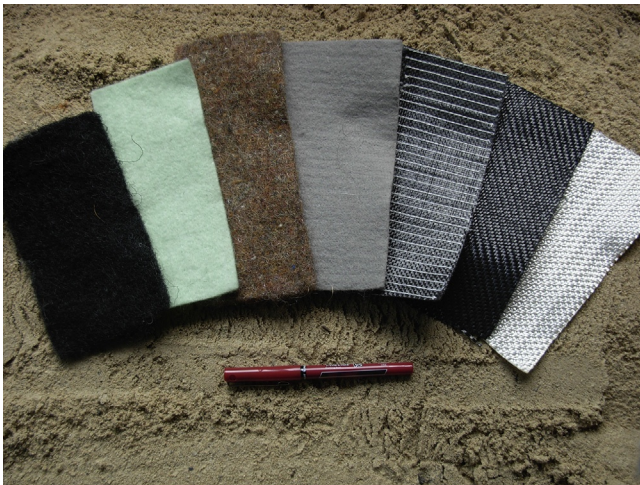
Figure 8.1 Photograph of a range of typical geotextiles used in geotechnical applications. Courtesy of Geosynthetic Institute.
