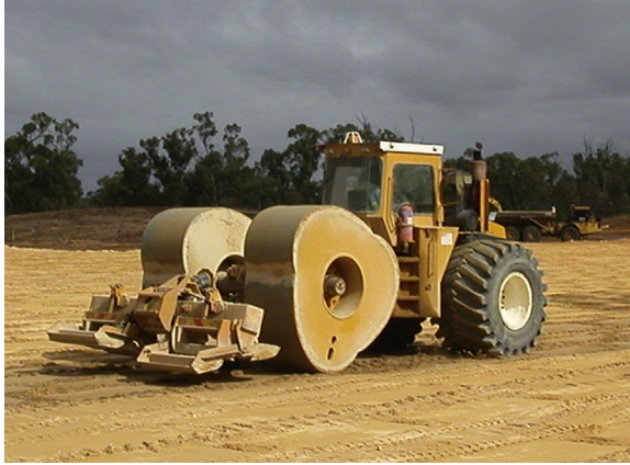
Figure 5.11 Impact roller. Courtesy of Landpac Technologies.
