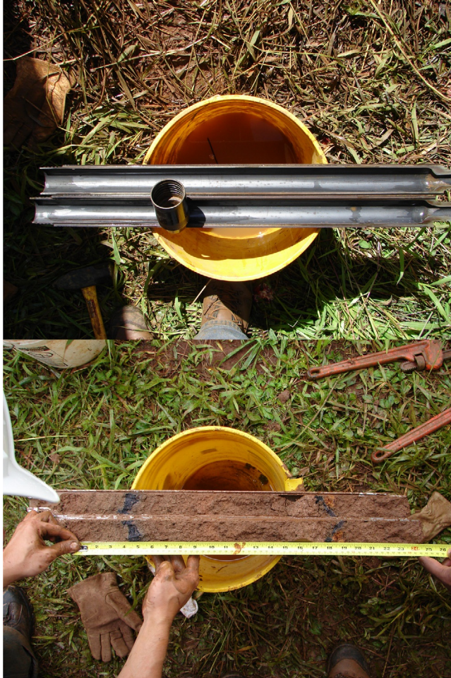
Figure 3.14 Split-spoon sampler empty and with a disturbed sample. Courtesy of Prof. Horst Brandes.
