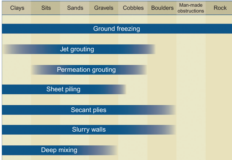
Figure 13.1 Freezing applicability compared to other improvement methods for ground support. Courtesy of Moretrench.
