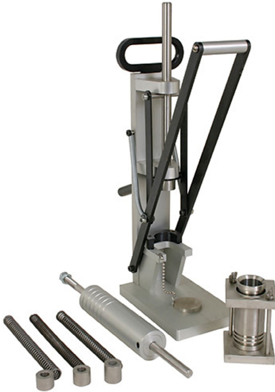
Figure 5.5 Harvard miniature compactor equipment.
