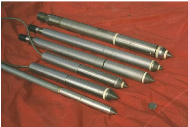
Figure 3.16 Assortment of cones used for cone penetration test. Courtesy of Prof. Paul Mayne.
