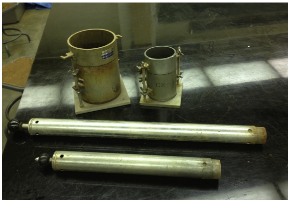
Figure 5.2 Standard and modified laboratory compaction hammers and molds.
