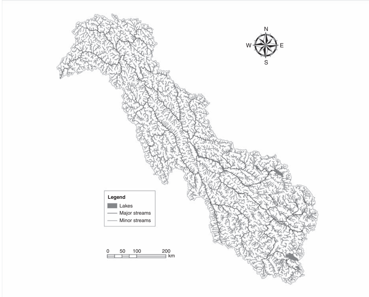
Fig. 2.7. The channel network of the Upper Indus Basin (UIB) derived from the digital elevation model (DEM). The major streams are marked with bold lines. A few lakes are also shown.
