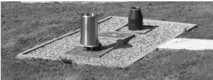
Fig. 2.2 Tipping bucket rain gauge (foreground) and storage gauge (background) in southern England. Photo: Y. Chen (Copyright © Environment Agency 2009 all rights reserved)
