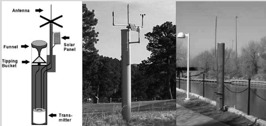
Fig. 2.9 Principles of operation of a radio-reporting raingauge (NOAA/NWS 2005) and illustration of an ALERT weather station and combined raingauge and streamflow gauge (Stewart 2009)
