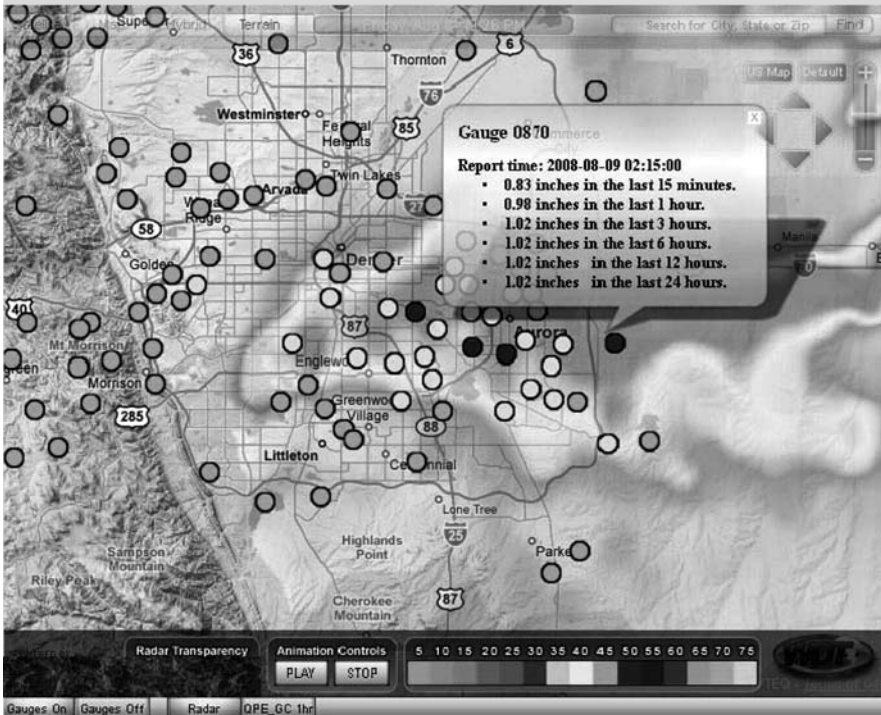
Fig. 2.10 Illustration of a combined internet based display of raingauge and NEXRAD weather data (Urban Drainage and Flood Control District, Denver, Colorado; Stewart 2009)
