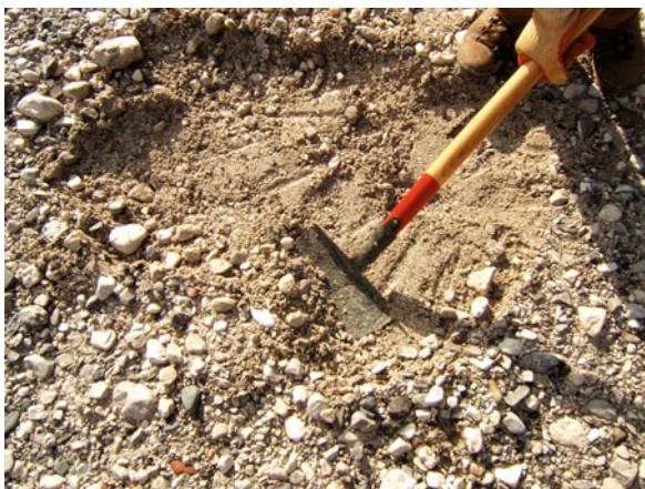
Fig. 13.5 Bulk sampling of the subsurface layer on the Na Belah gravel bar (933.7 km)
