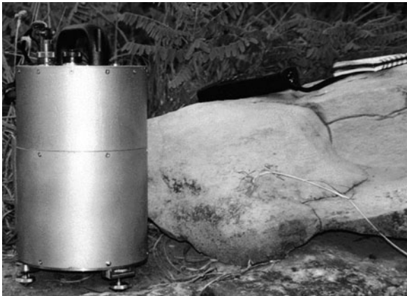
Fig. 3.3 Set up to measure ambient noise at a rock site just outside Duzce (Tromans, 2004)
