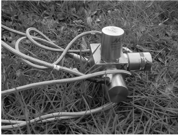
Fig. 7.37 The accelerometer arrangement used in the case study in Section 7.2.4.2
