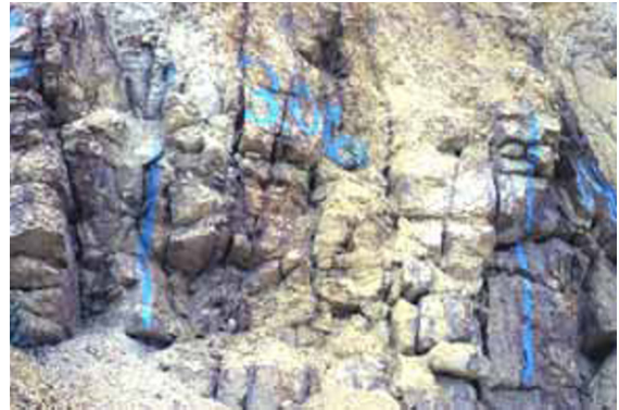
Figure 8.29. Vasil'kovskoe Au-As deposit, Kazakhstan. Closely spaced partly leached Au-arsenopyrite fractures in granodiorite (PL 8-1996). 3.06 (g/t Au) is the assay of this interval
