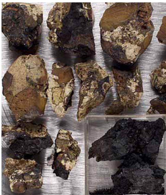
Figure 5.3. Cobaltiferous ferromanganese crusts ( black ) coating and filling cracks in bleached basalt of seamounts. White =biogenic CaCO 3 . Central Pacific, coll. J. Hein's group
