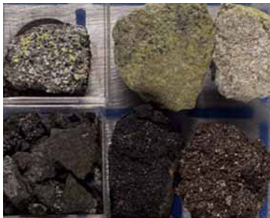
Figure 13.64. “Sandstone-U” ore, Ambrosia Lake deposit, New Mexico. Black, humate-impregnated coarse sandstone with dispersed coffinite, uraninite and U-humates. Top centre, secondary yellow U minerals form several weeks after exposure. Samples are about 4.5 × 3.5 cm, from LITHOTHEQUE
