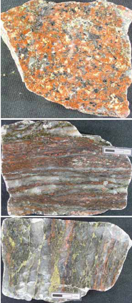
Figure 14.19. Malanjhand Cu–Mo–Au, India, lithology. 1. “Red” granite; 2, 3. Quartz stringers, veins and zones of silicification in sheared granitoids with stringer and disseminated Fe, Cu, Mo sulfides. Hand samples (~12 × 8 cm), from D. Kirwin’s collection, PL 1-2007
