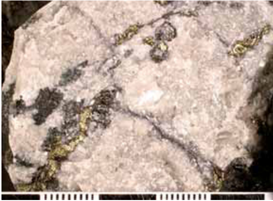
Figure 12.35. Blebs and patches of chalcopyrite and bornite with magnetite in transgressive carbonatite; Palabora, South Africa. (scale in cm, from LITHOTHEQUE)
