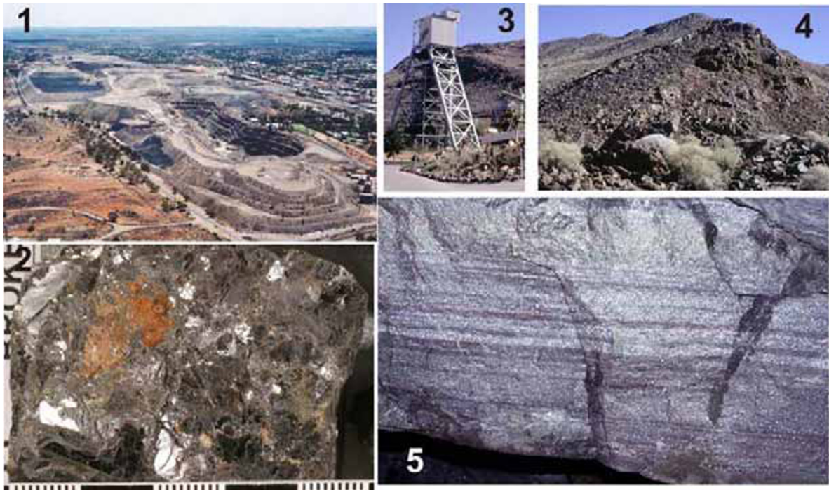
Figure 14.9. Broken Hill, NSW and Aggeneys photos, 1. Central Broken Hill open pits on site of former shafts, looking east; 2. Coarse recrystallized massive galena, sphalerite ore; 3. Aggeneys, Broken Hill Shaft; 4. Aggeneys, Black Mountain Lode outcrop marked by a ridge of adjacent siliceous BIF; 5. Aggeneys, Broken Hill banded densely disseminated sphalerite, galena in quartzite gangue. Photo 1 courtesy of Consolidated Broken Hill Ltd., # 3–5 PL 1991, #2 from LITHOTHEQUE. Sample 2 is about 5 \times 4 cm, #5 about 2 \times 1 m
