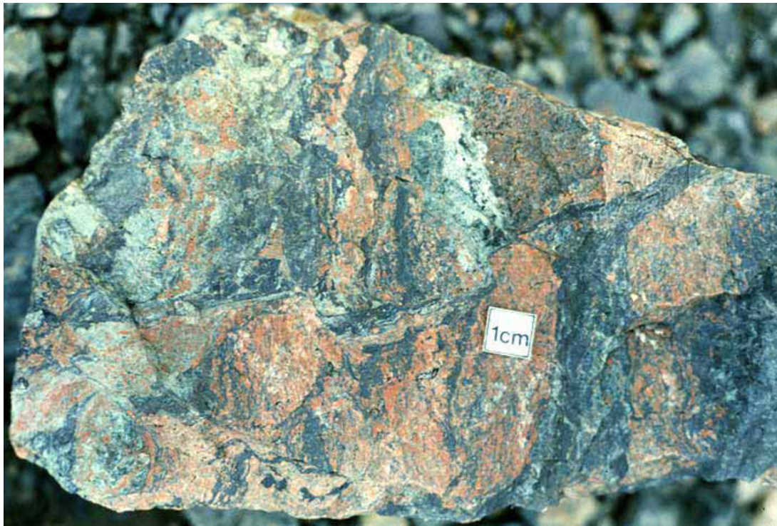
Kiruna, Per Geijer hematite orebodies. Breccias of progressively albitized sandstone fragments partly replaced by hematite. PL 2006.
