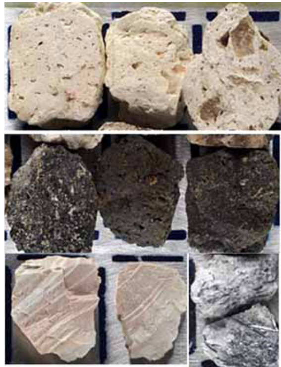
Figure 6.15. Hot springs lithology. Top row shows silica residue after complete leaching of andesite (middle row) by hot springs at Sulfur Bank (LITHOTHEQUE 1156). Bottom row shows banded opaline sinter (two on left) and quartz-stibnite gold ore from the McLaughlin Mine (LITHOTHEQUE 1829). Each sample is about 3.5 × 4.5 cm
