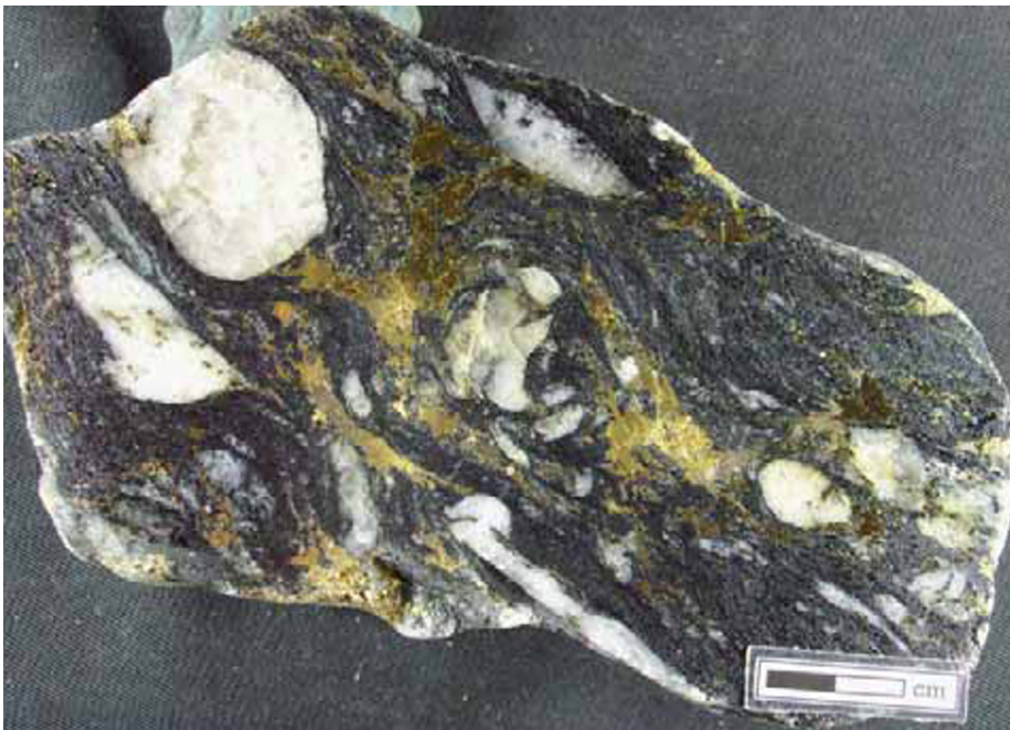
Metamorphic ore structures. Top: Thompson Ni, Manitoba, Canada. Mixed “ball” and “pegmatite” ore. Ball ore is a ductile breccia of brittle rock fragments “floating” in a paste of ductile pyrrhotite and pentlandite injected by synorogenic pegmatite that soon broke to yield breccia fragments. Bottom: Cu ore breccia, Mosaboni Mine, Singhbhum Belt, Jharkhand State, India. Brittle partly rotated quartz fragments embedded in phyllonite with chalcopyrite stringers. PL 1983, 2008; Mosaboni sample is from D.Kirwin’s collection. Scale bars 1 & 2 cm, respectively.
