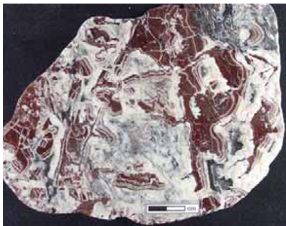
Figure 11.41. Beltana (Puttapa), a medium-size oxidic Zn deposit in the Flinders Ranges of South Australia. Breccia of older (red) hematite-pigmented willemite is cemented by white drusy willemite. PL 1-2007, from D. Kirwin's collection
