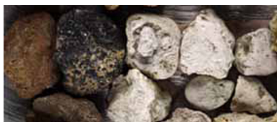
Figure 13.33. Florida “land pebbles”, relatively fresh (honey yellow), incrustated with Fe–Mn hydroxides, and leached (chalky white). 10 cm across. Fort Meade, from LITHOTHEQUE
