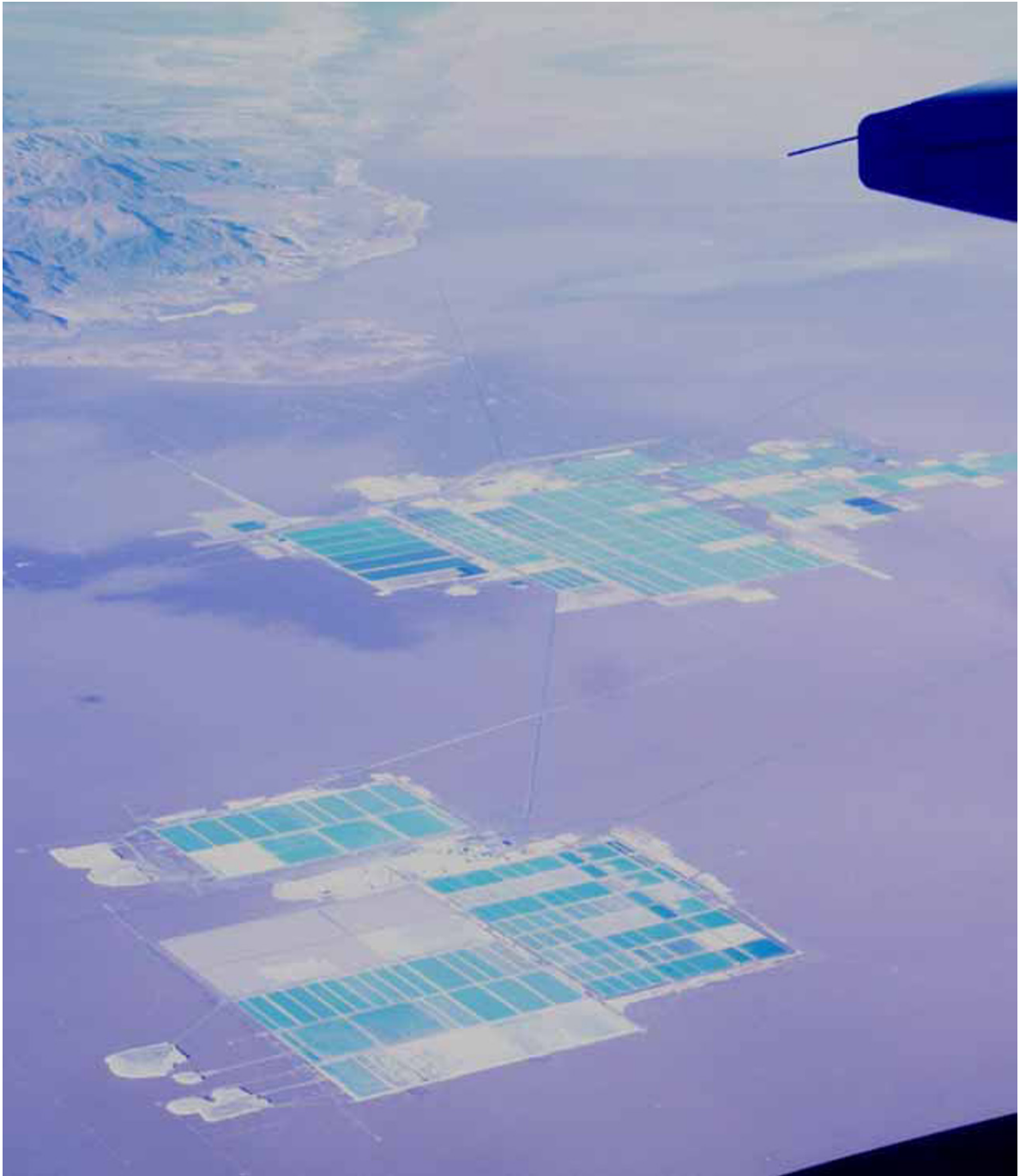
Unconventional resource exploitation: Salar de Atacama lithium operations, based on evaporation of playa brine. PL 4-2009
