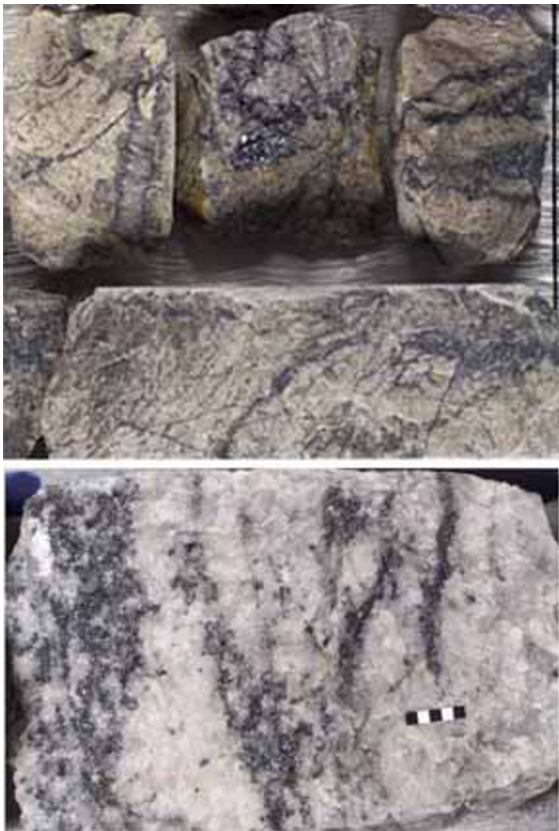
Figure 7.55. Distinct appearance of the Climax-type molybdenite-only fracture stockwork and diffuse schlieren of moly in silicified porphyry. Henderson, Colorado, from LITHOTHEQUE. Scale bar=1 cm
