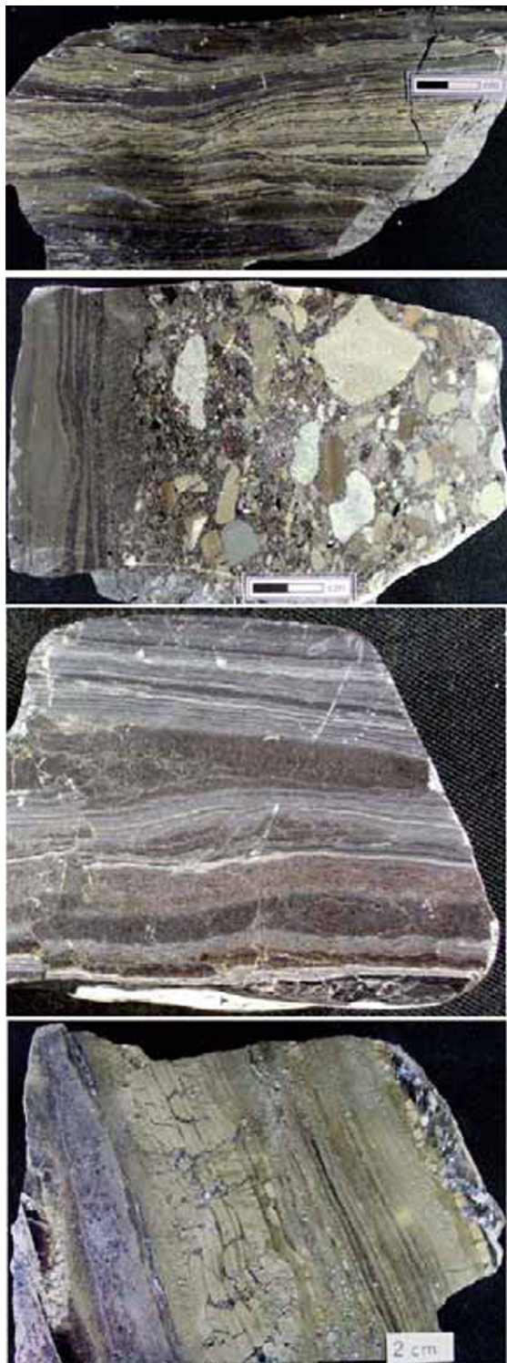
Figure 11.6. Sedex ore slabs, Mt. Isa Inlier. 1, 2, McArthur River HYC deposit; pyrite, sphalerite, galena finely banded ore, slight syndepositional deformation. Sample #2 has heterolithic debris flow breccias impacting banded ore. 3. Century mine, banded sphalerite > galena, interlaminated “black shale”;
