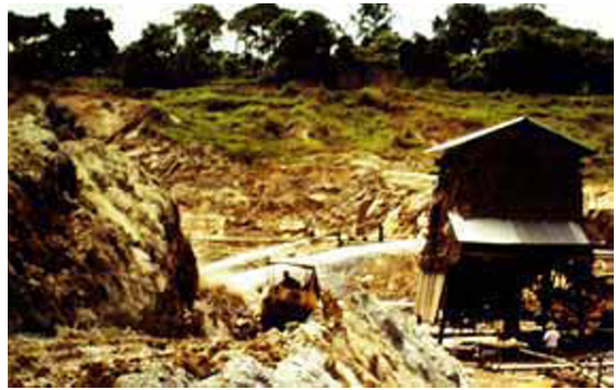
Figure 13.53. Tin pit (now reclaimed) near Kuala Lumpur with water monitoring of the soft “eluvial placer” (=argillized tin granite with residual cassiterite) under way. PL 1980
