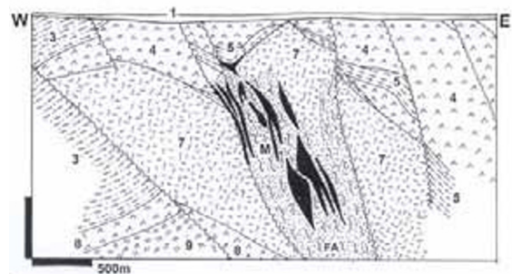
Figure 9.13. Gai (Gaiskoe) VMS ore field, southern Urals, Russia, from LITHOTHEQUE 4105 modified after Pavlova et al. in Prokin, et al., (2004). M. D 1 Urals-type complex multistage massive and disseminated Fe, Zn, Cu sulfide system. 1. Q cover & regolith; 3. D 2-3 back-arc basalt & sediments; 4. D 1-2 arc basaltic andesite; 5. Ditto, volcanoclastics; 7. D 1 andesite, dacite, rhyolite stratovolcano facies; 8. Ditto, metabasalt & hyaloclastite; 9. Rhyolite, dacite
