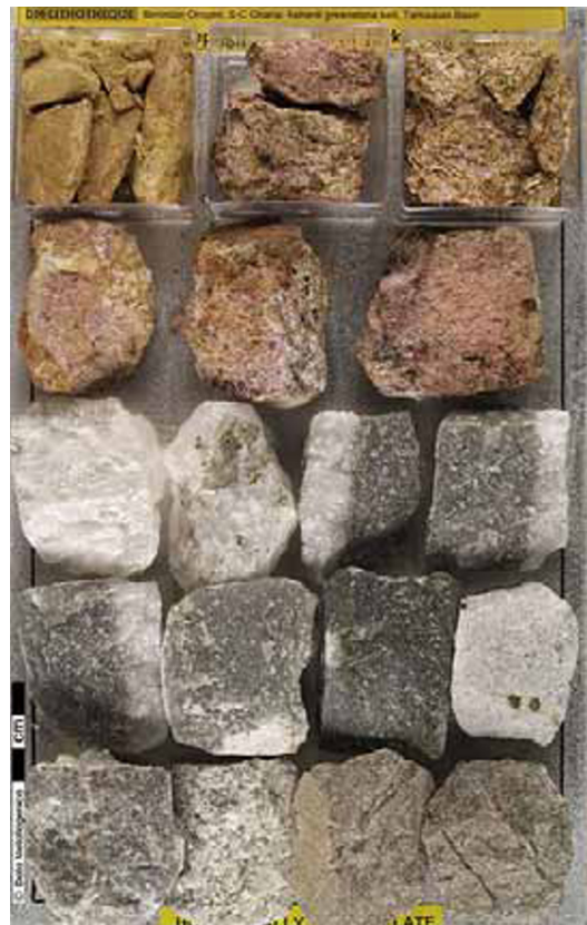
Figure 10.45. Damang Au deposit, Tarkwa goldfield, LITHOTHEQUE plate 2796, showing the oxidized Au ore in leached conglomerate (top) and the primary quartz-veined clastics (bottom)
