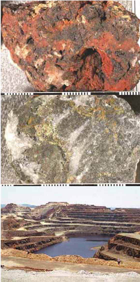
Figure 9.22. Rio Tinto, Cerro Colorado Au-bearing gossan (top), pyritic footwall stockwork under VMS orebody (center), and flooded open pit (PL 8-2001)
