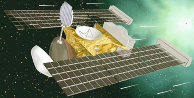
■ Artist's impression of NASA's Stardust spacecraft approaching comet Wild-2. Note the tennis-racket-shaped, aerogel-filled dust particle collector which was deployed to catch microscopic dust particles from the comet's coma. Image courtesy of NASA Jet Propulsion Laboratory.
