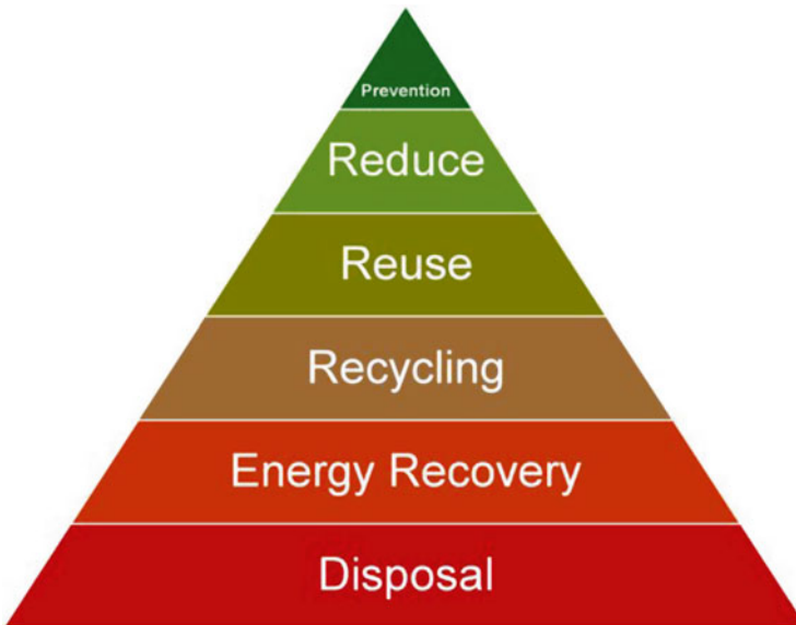
Fig. 12.4 The waste disposal hierarchy. The relative carbon footprint of waste disposal is shown at the base of the pyramid. Recycling, energy recovery and disposal are the least environmental friendly options in that order with the options with the lowest footprint at the top
