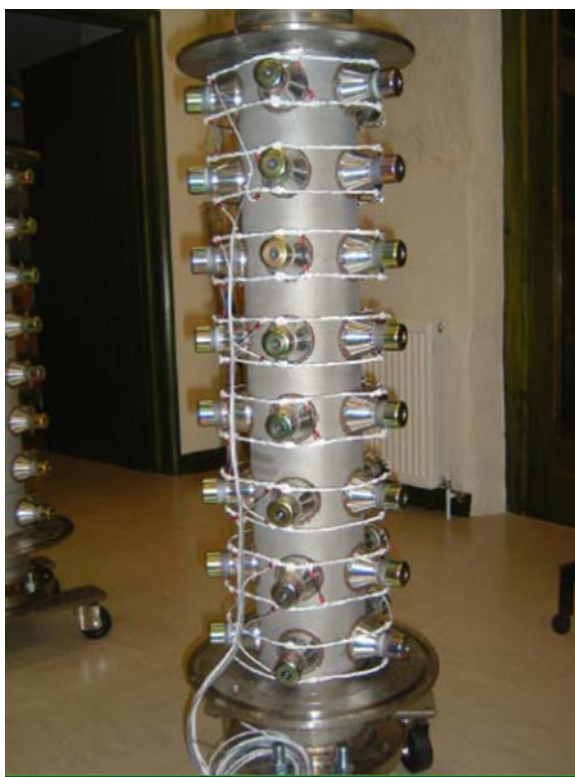
Fig. 2.8 A 20 L Prosonitron multiple 20 kHz bonded transducer flow cell (WO 00/35579). Photograph courtesy of Prosonix Ltd, UK, www.prosonix.co.uk
