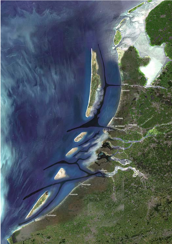
Fig. 3.20 Row of islands in front of the Western Netherlands coast (Source: Boskalis, 2008)
