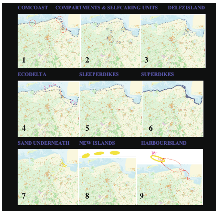
Fig. 3.25 Nine new solutions for the Groningen coastal defence (Source: Province of Groningen & Climate Changes Spatial Planning, 2008)
