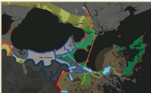
Figure 15. Lake Pontchartrain Barrier Alignment: #3-Lake Borgne.
