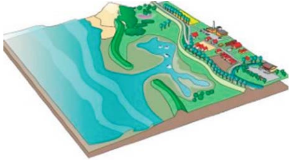
Fig. 3.11 Back draw of the dike (Source: Oedekerck, 2006)
