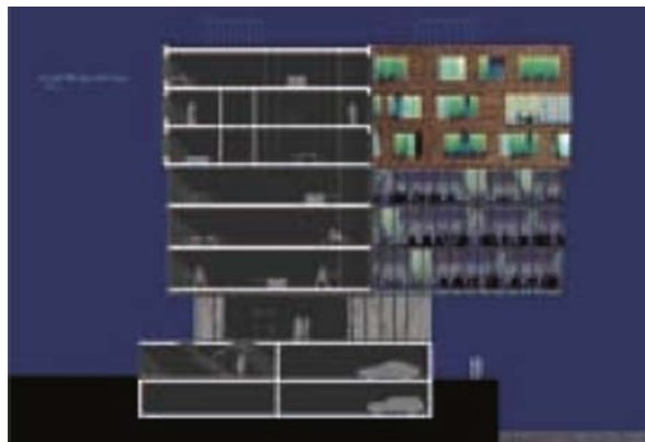
Fig. 3.38 Examples of buildings above exceptional flood levels (Source: GHS, 2002)
