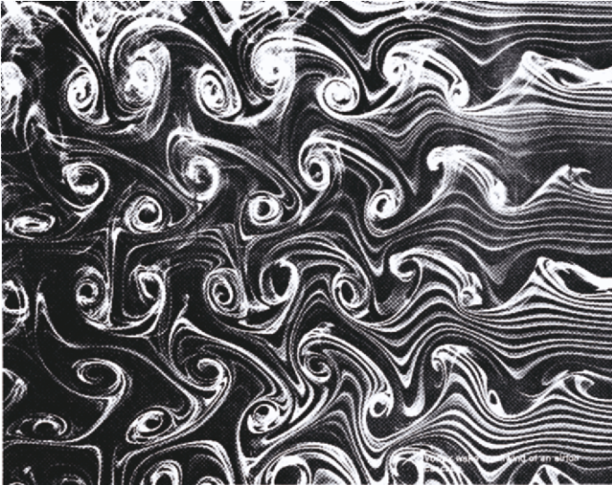
Figure 1.18: Evidence for the intense vorticity within any canopy layer (permission to publish of Prof. J. Cermak, Colorado University, USA is kindly acknowledged).
