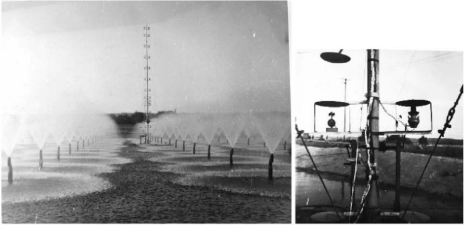
Figure 1.13: Gradient mast within spraying system (A) and the measurement unit of a remote anemometer (left) and a psychrometer (right) on it (B) used in the field investigations within a SCS [209, 217].
