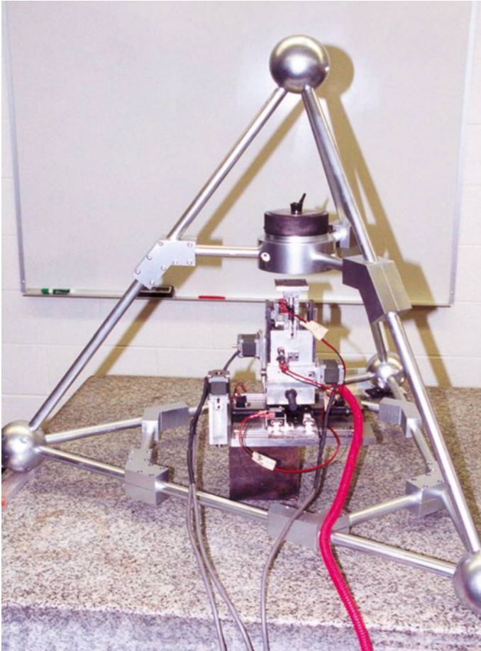
Fig. 7.7 Piezoelectric machining center capable of nanogrinding. Re-printed with kind permission from Springer Science+Business Media B.V.
