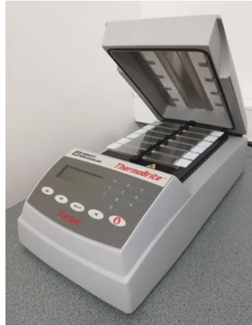
Fig. 4 ThermoBrite apparatus recommended for FISH. Complete specifications for this can be found at http://www.leicabiosystems.com/ihc-ish-fish/ish-probes-molecular-pathology/kreatech-fish-probes/equipment/thermobriter/
