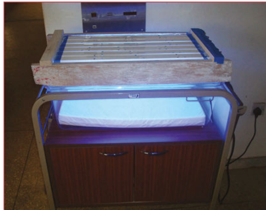
Figure 20-16. Phototherapy Device Constructed for Use With a Bassinet (Note Extended Spacing Bars for Protection of Lamps)
