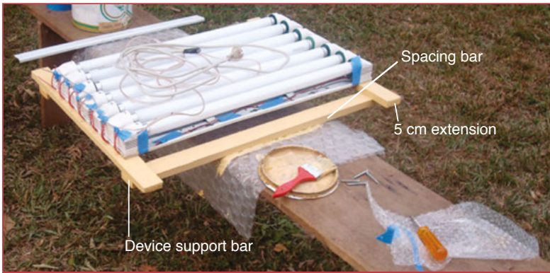
Figure 20-13. Assembling a Locally Made Phototherapy Device
