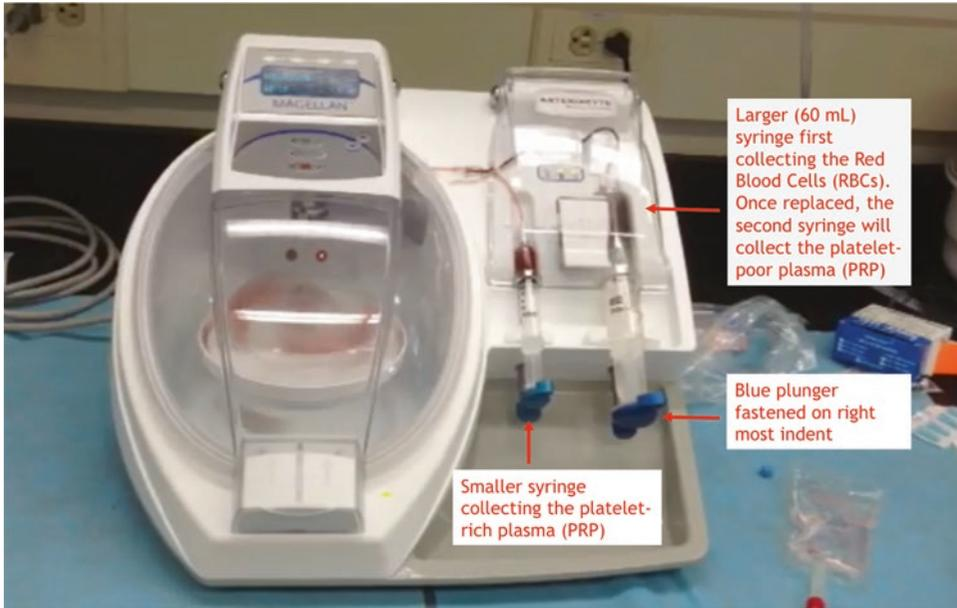
**Fig.2** Magellan® System used to process human peripheral blood—it is a completely automated and close-looped device with the ability to separate blood into three fractions: red blood cells, platelet-rich plasma, and platelet-poor plasma. The latter fraction was used to form fibrin gel by mixing with an appropriate amount of calcium chloride solution
