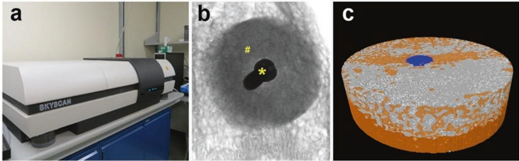
**Fig. 4** Micro-CT analysis. (a) SkyScan 1172 micro-CT scanner. (b) 2D X-ray projection showing three materials with different X-ray attenuations: titanium screw (\*), biomaterial (#), and rabbit bone. (c) 3D reconstructed micro-CT image using CTAn software showing three materials demonstrating a titanium screw (*blue*), the biomaterial (*orange*), and the rabbit bone (*light gray*)
