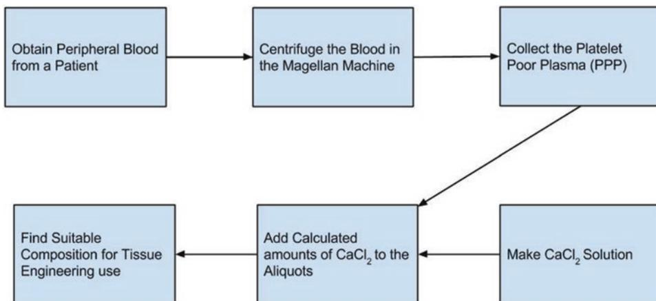
**Fig. 1** Schematic showing the steps utilized to prepare fibrin gel from human blood-derived plasma. Plasma was obtained by processing peripheral blood via Magellan<sup>®</sup> System followed by calcium-mediated gelation
